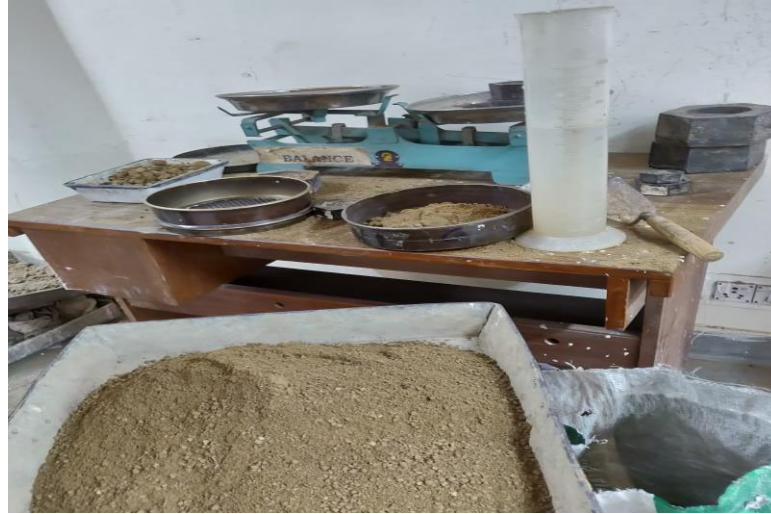
Figure 4.5 Dry soil for CBR test mould
