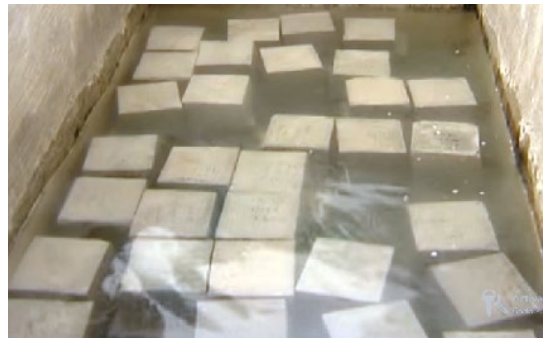
Figure 4.5 Curing of Concrete Cubes
