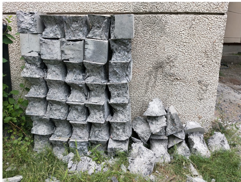
Figure 5.1.5 Failure of Concrete cubes
