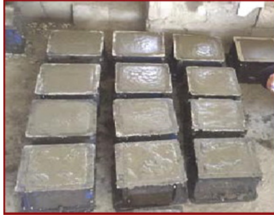
Figure 4.4 Casting of Concrete cubes
