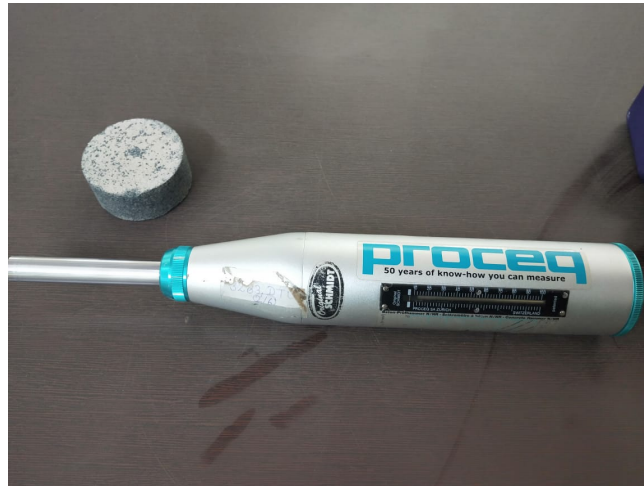
Figure 5.1.2 Proceq Rebound Hammer Apparatus
