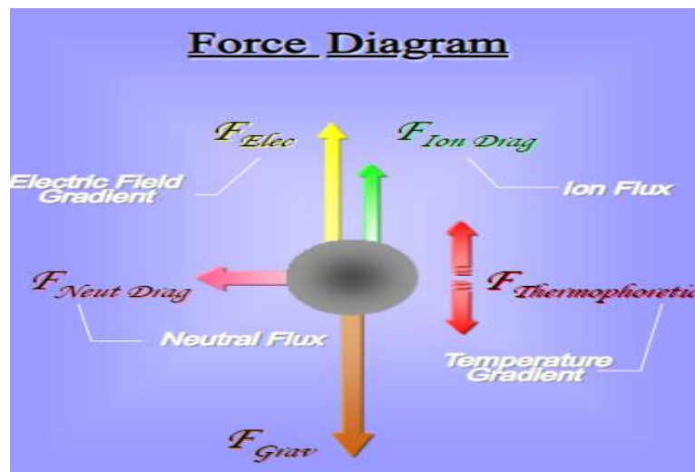
Fig. 1.2 Different forces acting on dust grains floating in plasma [11]
