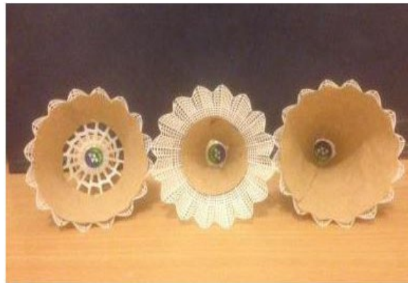
Figure 6: Modified synthetic shuttlecock with upper, lower, complete skirt covered [7].
