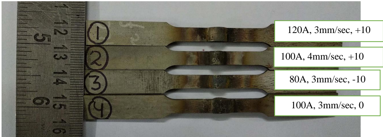
Figure 5.7: Test specimens for tensile testing taken from UCMT welded samples
