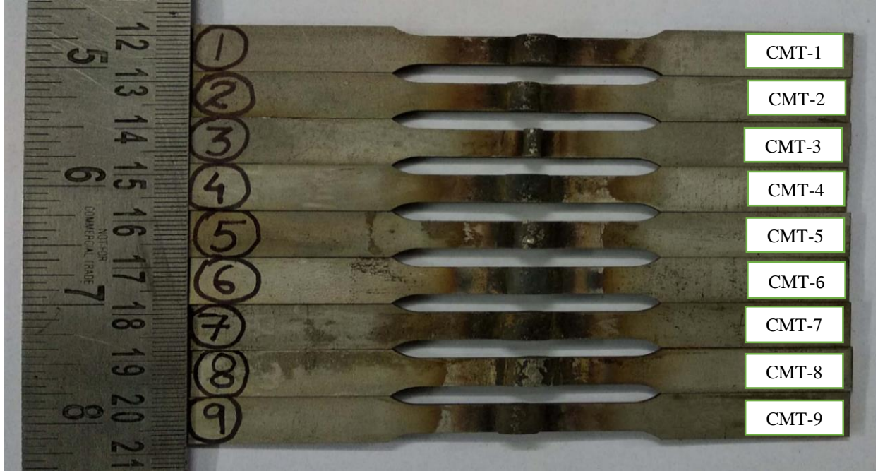
Figure 3.13: CMT welded specimens test specimens for tensile testing
