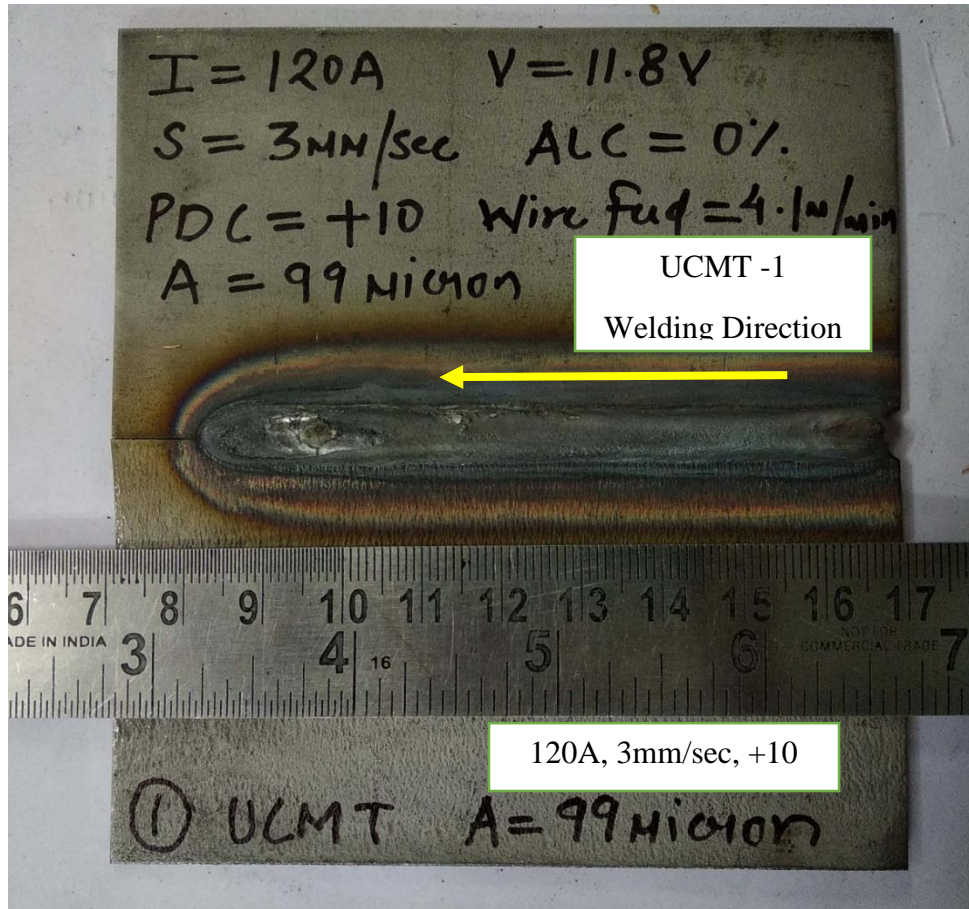
Figure 5.3: Image of UCMT welded SS 202 of thickness 1.58 mm at Current 120A, Welding Speed 3mm/sec, and Pulse dynamic correction Factor +10
