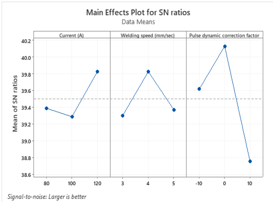
Figure 4.7: Mean S/N ratio graph for Yield strength (MPa), Ultimate tensile strength (MPa), Percentage elongation (%)
