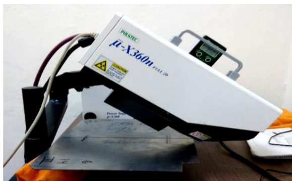
Figure 18 Portable X-ray machine ( \mu -X360) using measurement of Residual stress in Precision Lab
