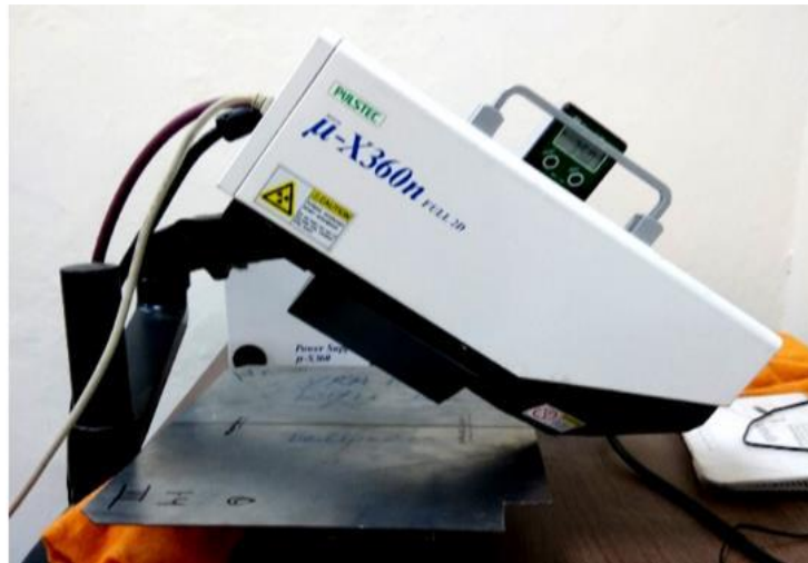
Figure 16 Portable X-ray machine ( \mu -X360) using measurement of Residual stress in Precision Lab
