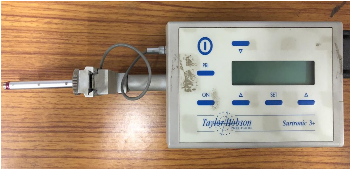
Figure 5 Surface roughness measurement instrument in Metrology Lab
