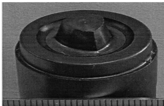
Figure 8: Design of thread less pin [3]
