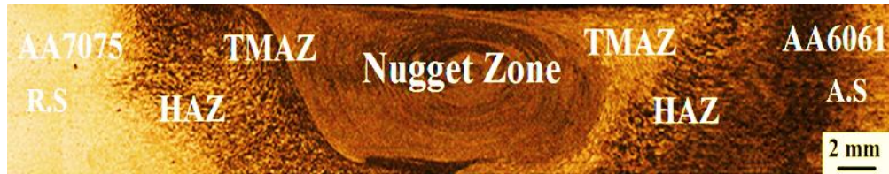
Figure 98: Macrostructure of the TIG+FSP welded joint of AA6061 and AA7075
