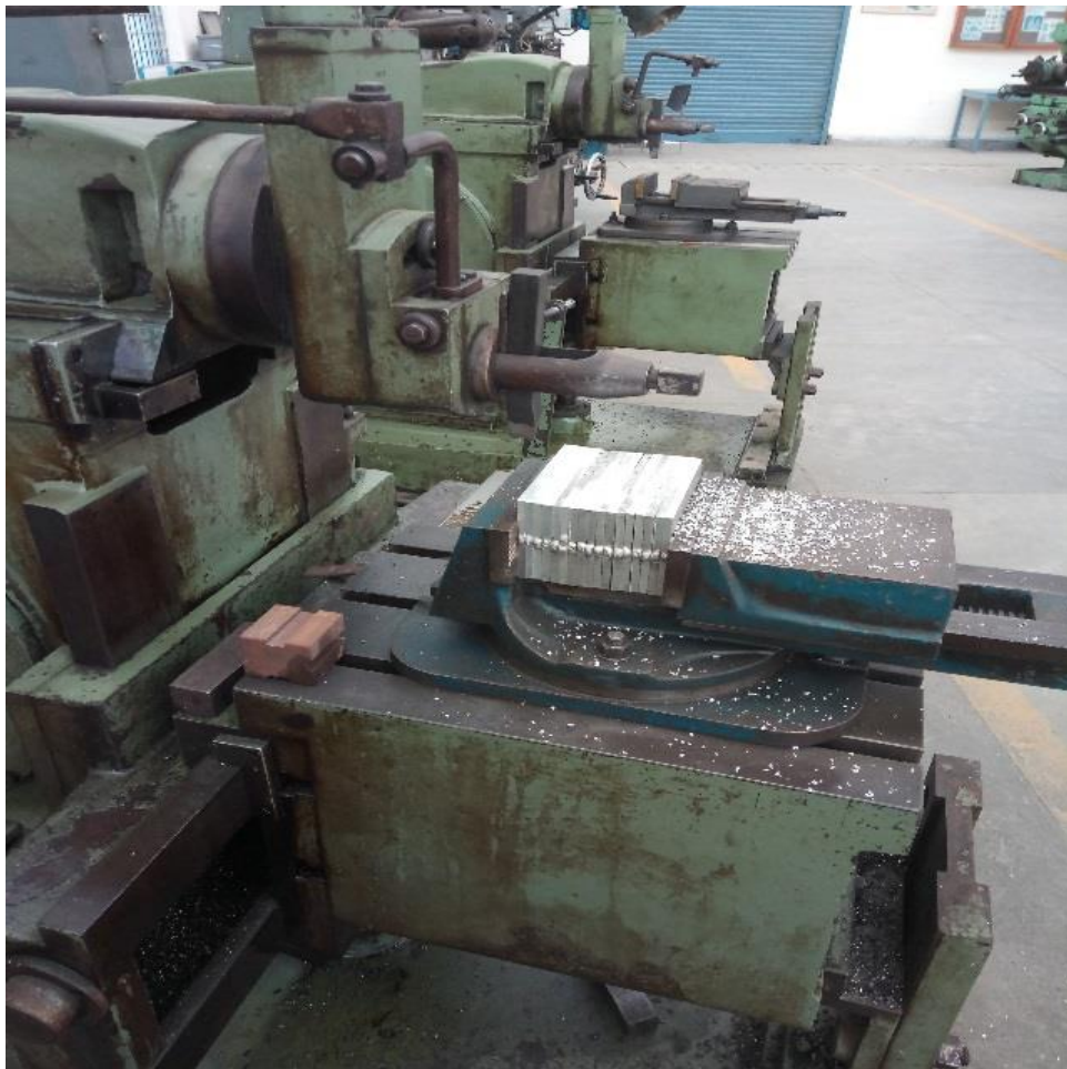
Figure 35: (a) TIG+FSP welded joint, (b) Strip from welded joint, (c) Tensile test specimens as per ASTM E8, (d) Tensile test specimen dimensions, (e) finishing of welded plate by shaper
