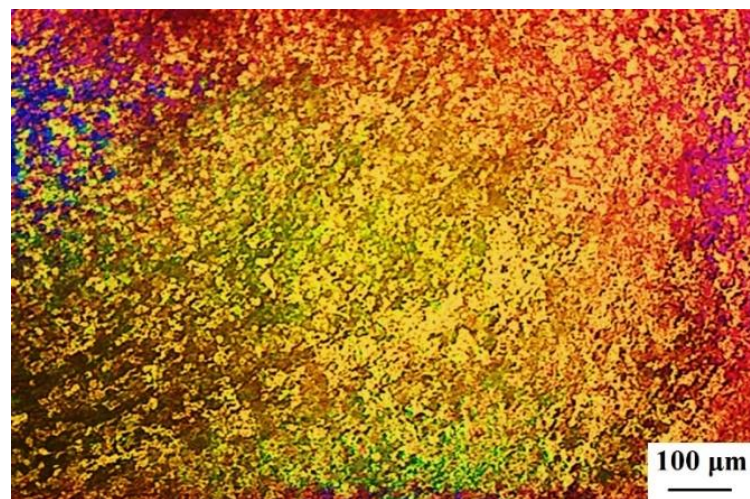
Figure 98: Macrostructure of the TIG+FSP welded joint of AA6061 and AA7075
