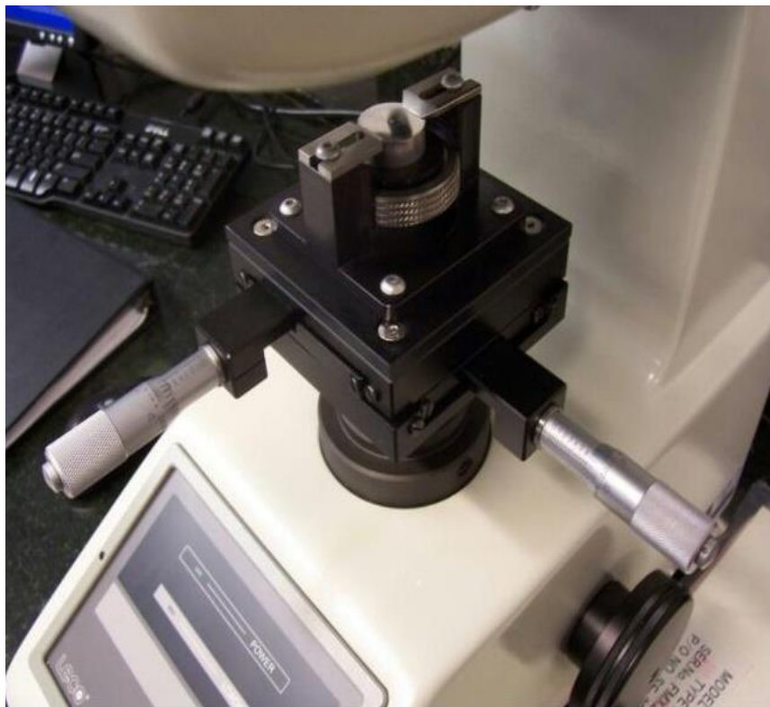
Figure 37: Vickers micro hardness testing process
