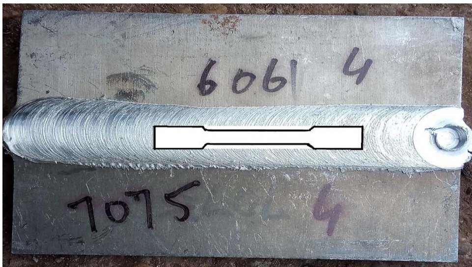
Figure 72: (a) Dimension of TIG+FSP welded tensile specimen, (b) Tensile specimen along the welding direction
