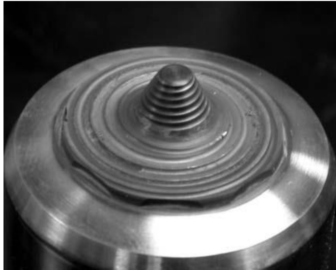
Figure 5: Design of round bottom cylindrical pin [3]
