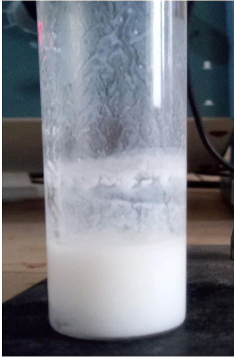
Figure 12 : BSA nanoparticle solution after adding ethanol dropwise and cross-linking agent, glycerol.
