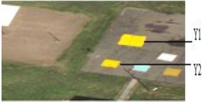
Figure 3.1: Mixed pixel target Y1 and full pixel target Y2 in subset S2
