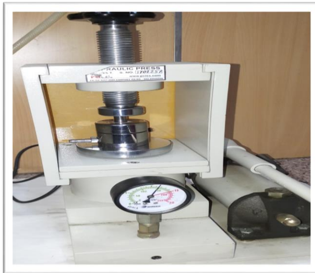
Figure 3.8.2: Hydraulic pump system for pellet preparation
