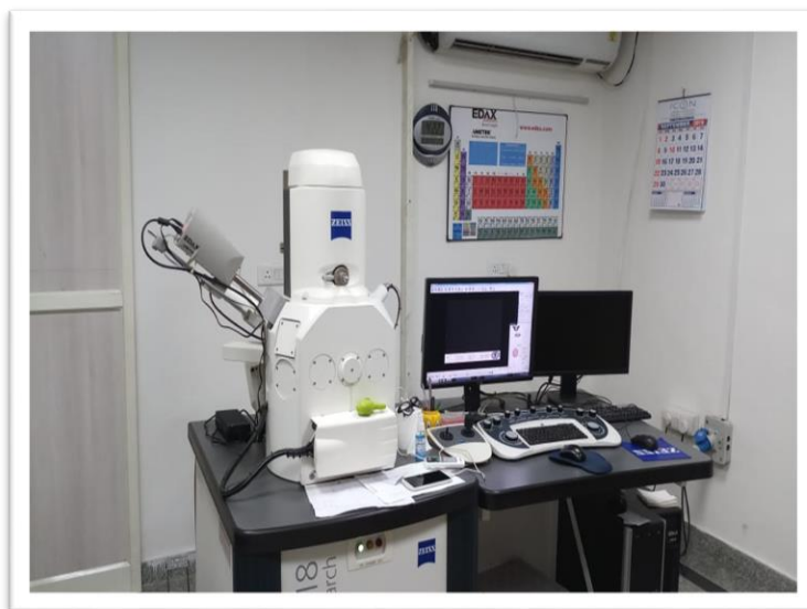
Figure 3.5: SEM system EVO18 Zeiss for determining surface morphology (New York, USA)
