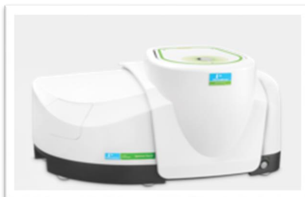
Figure 3.2.1: Perkin Elmer Spectrum 2 FTIR system for estimation of functional groups (USA)
