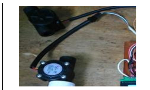
Figure 13: Flowrate sensor/Flow meter
