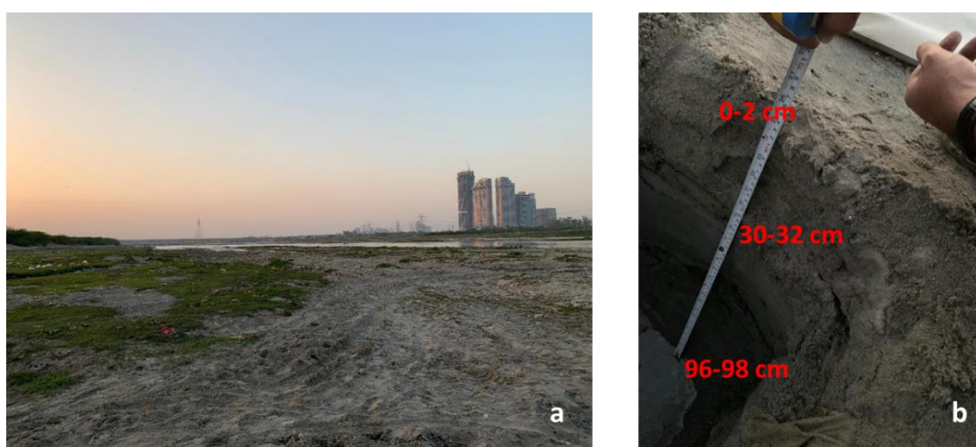
Fig. 3.3: (a) SITE B Okhla barrage, Yamuna river bed, (b) sample collection from river bed.
