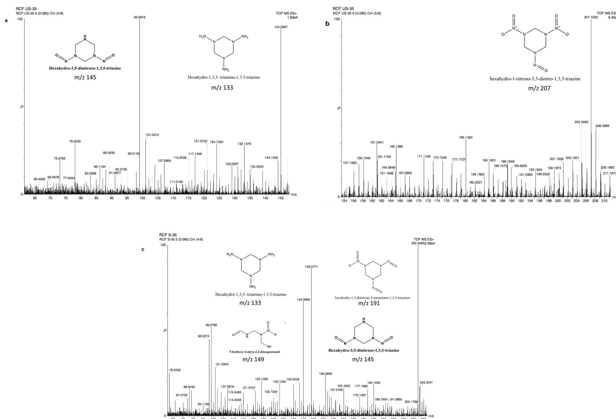
Fig. 6. MS chromatogram for RDX degradation under (a & b) unsaturated and (c) saturated conditions.
