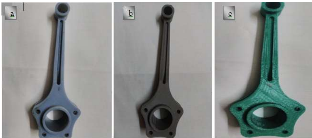
Figure 3.4: Fabricated prototype model of connecting rod (a) Objet30 (PolyJet) printer. (b) MakerBot (FDM) printer (c) Ultimaker (FDM) printer.
