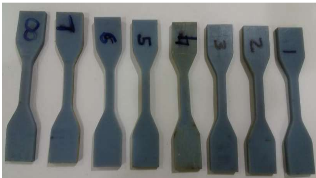
Figure 5.5: Fabricated ASTM D638 tensile test specimen
