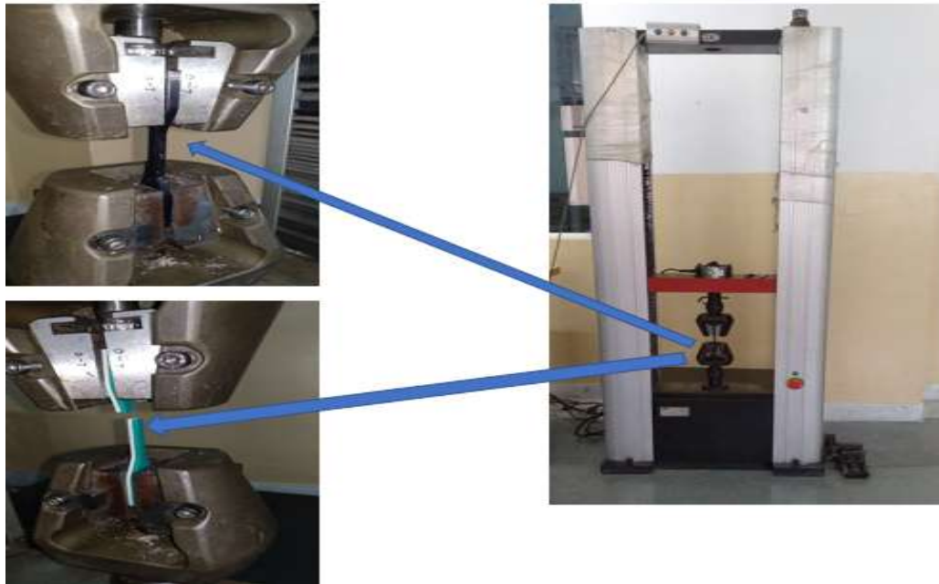
Figure 6.7: UTM Instron tensile testing machine
