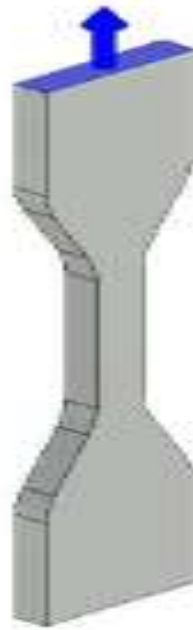
Figure 6.11: Loading condition of the test specimen
