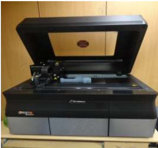
Figure 3.1(a): Experimental setup of PolyJet machine
