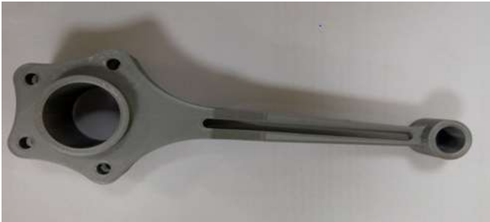
Figure 4.4: Prototype scaled model of connecting rod fabricated through the FDM process
