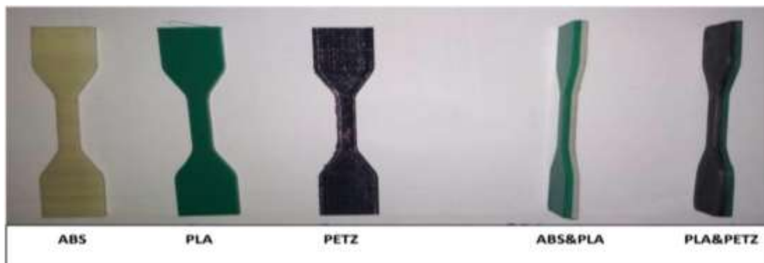
Figure 6.6: Fabricated specimen along the flat orientation
