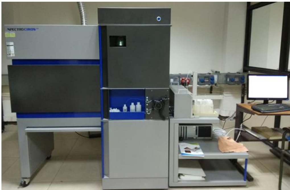
Figure 3.4.3: (b) SpectroCiros ICP-OES used for the analysis of As, Ni and Pb
