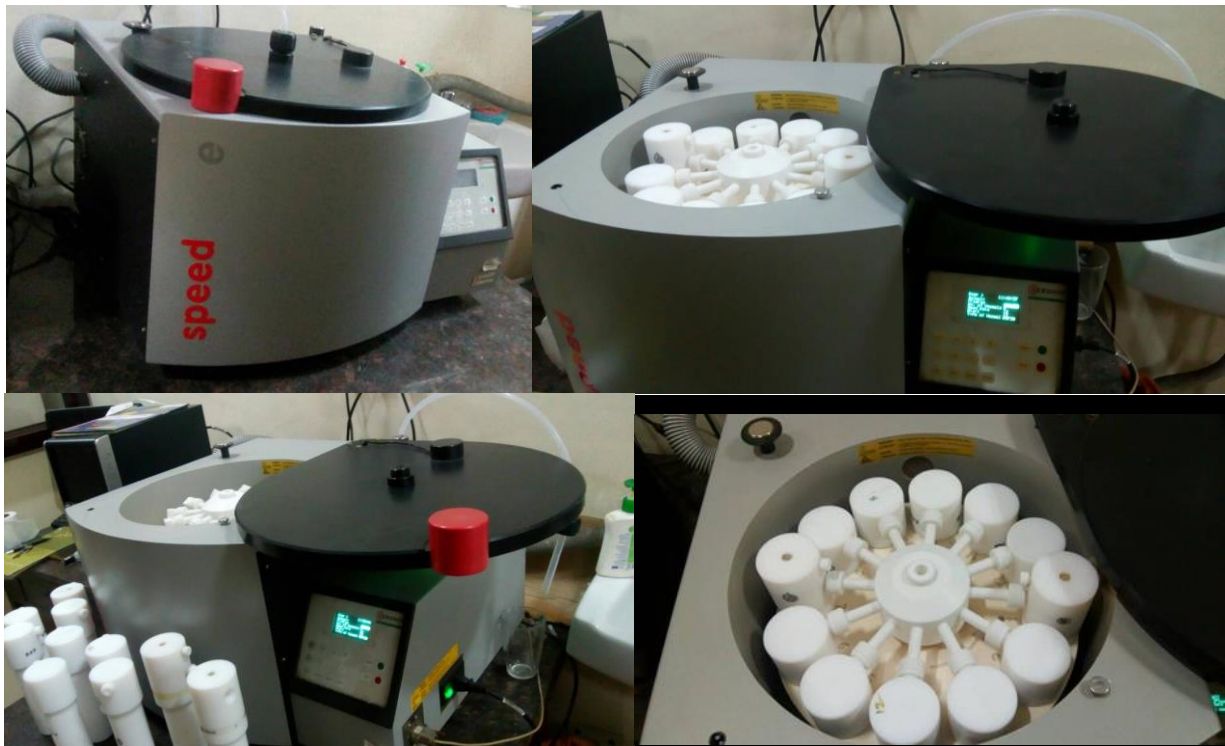
Figure 3.4.2: Speedwave Bergohf Microwave digestion system used for acid digestion for analysis of As, Ni and Pb in PM 10 samples
