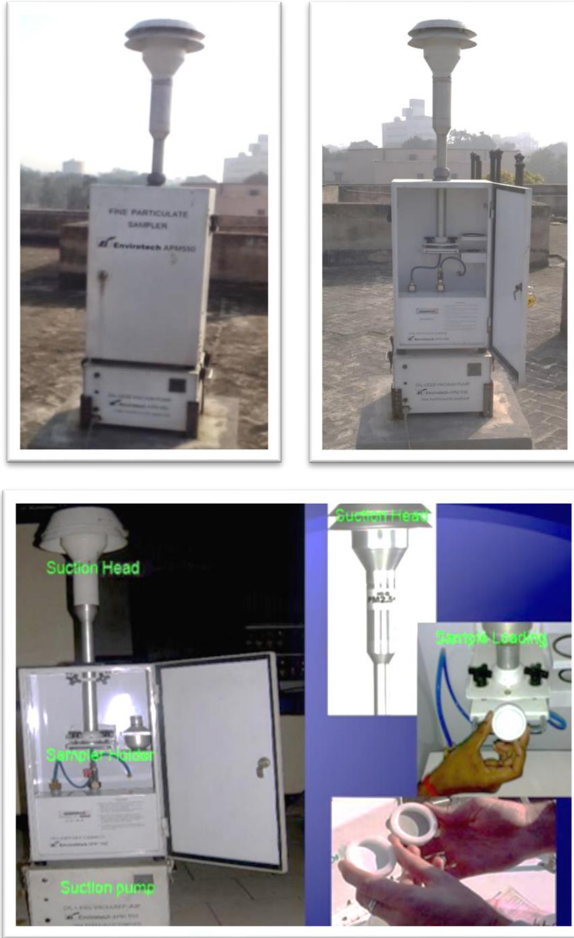
Figure 3.2: Envirotech APM 550 installed at NPL, New Delhi used for sampling of PM 10
