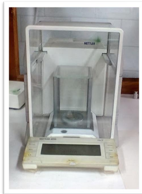
Figure 3.3: (a) Mettler-Toledo AX105 (range 0.1-100 mg) balance used for weighing PM 10 filters and metal standards and (b) Mettler AT20 (range 0-22g) balance used for the standard preparation of BaP
