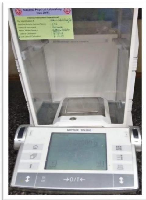
Figure 3.3: (a) Mettler-Toledo AX105 (range 0.1-100 mg) balance used for weighing PM 10 filters and metal standards and (b) Mettler AT20 (range 0-22g) balance used for the standard preparation of BaP
