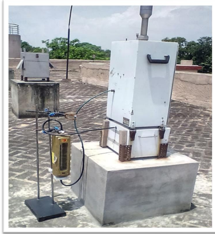
Figure 4.2: Schematic representation of the measurement of the flow rate during the sampling of PM 10
