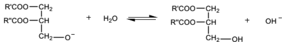
Figure 2.19: Alkali-catalysed transesterification reaction [169].
