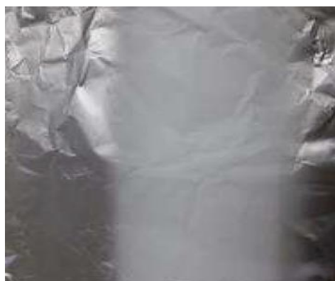
Figure 4.11 100% PVA (9% w/v) electro spun web
