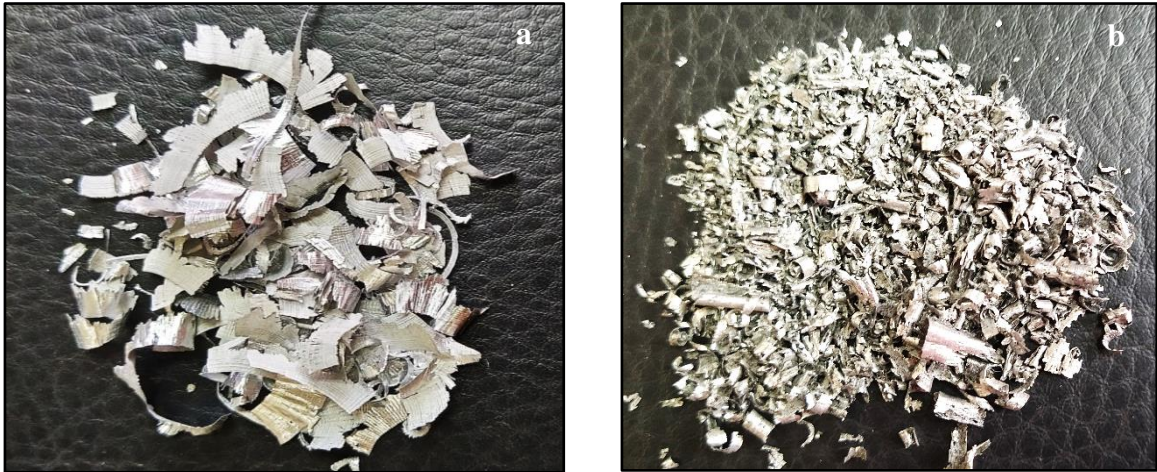
Figure 7.4: Chips Formed During Machining of (a) As-cast Al7075-T6 (b) Aluminium Composites
