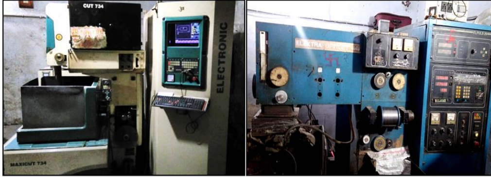
Figure 4.17: Wire Cut EDM for Standard Specimen Fabrication
