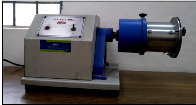
Figure 4.6: Ball Mill used for Preparation of Eggshell Powder
