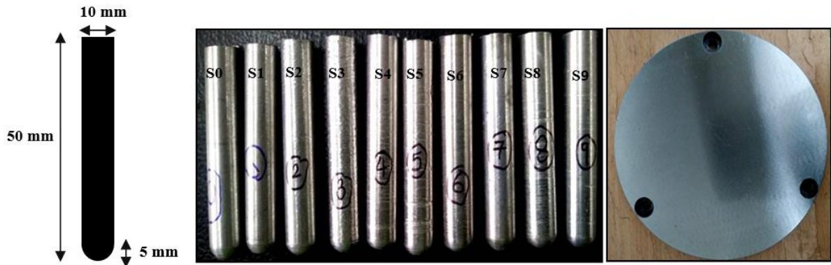
Figure 4.21: Standard Wear Test Specimens as per ASTM G99-17 and EN 31 Disk
