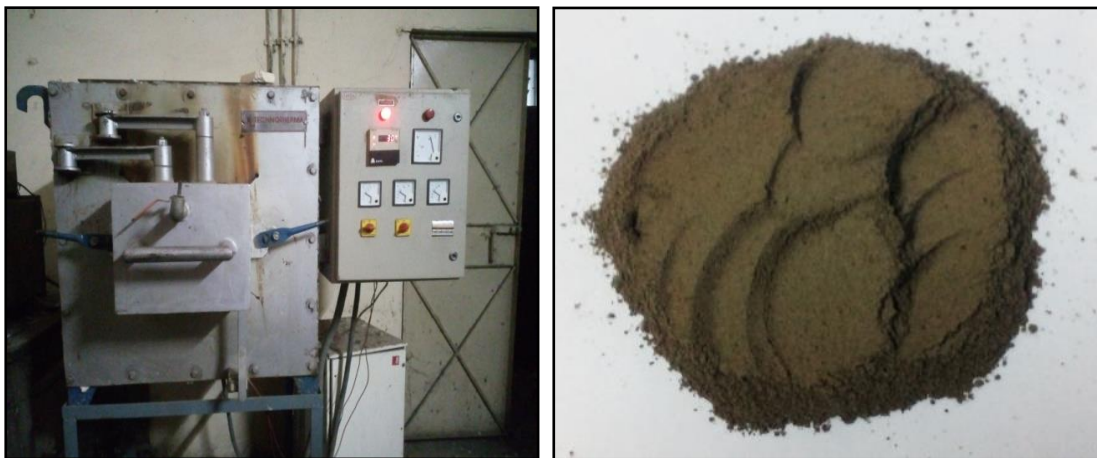
Figure 4.7: Muffle Furnace and Carburized Eggshell Powder
