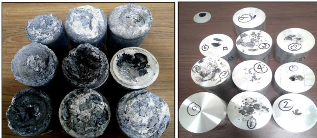
Figure 4.16: Solid Castings (One as-cast Al7075-T6 and Nine Hybrid Composites)
