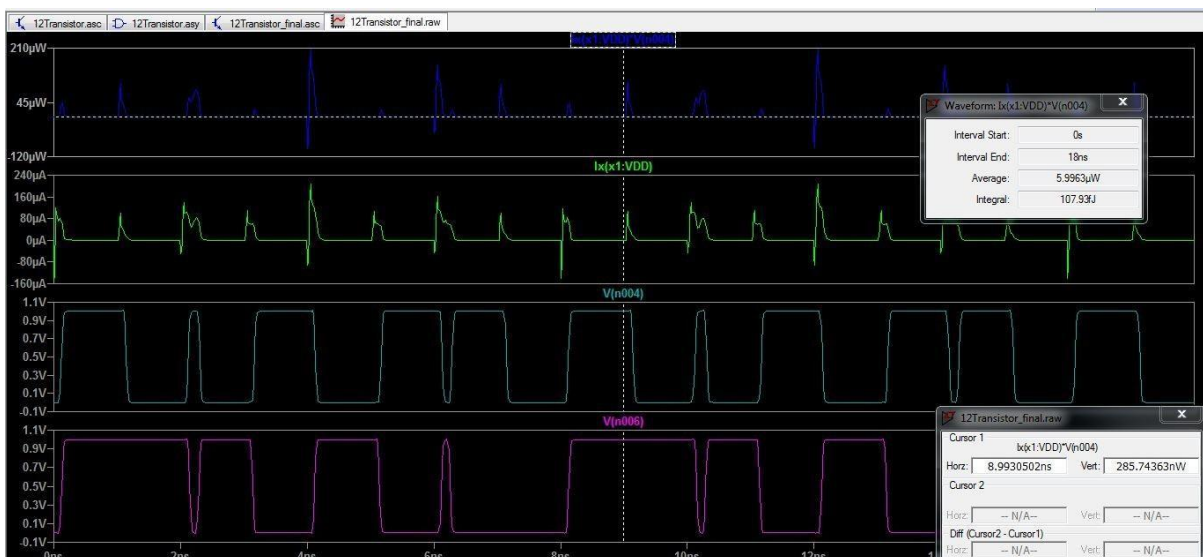
Figure xli. LT Spice 12 Transistor Full Adder Power Sum Graph
