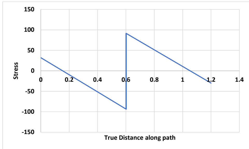
Figure 5.37. True distance along cross section vs in residual stress of AA5083 at 30°C
