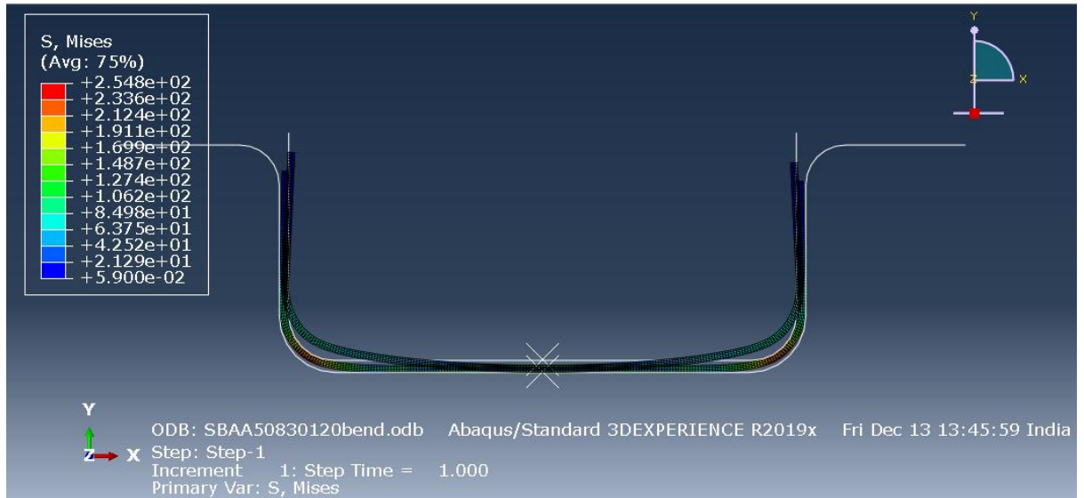
Figure 5.19. overlay plot showing springback of AA5083 at 120°C
