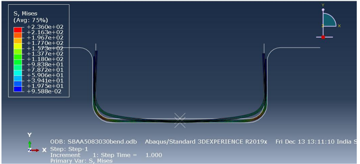
Figure 5.17.overlay plot showing springback of AA5083 at 30°C
