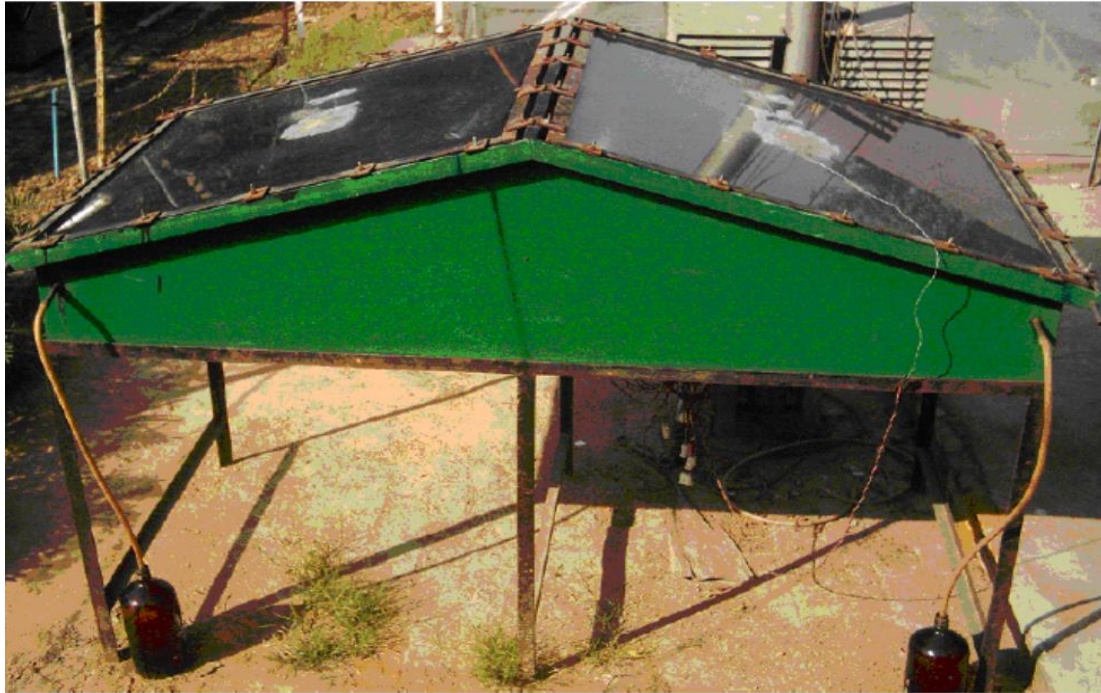
Fig. 1.5. Double slope passive solar still at I.I.T Delhi
