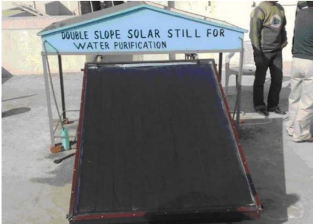
Fig. 1.6. Double slope active solar still [25]
