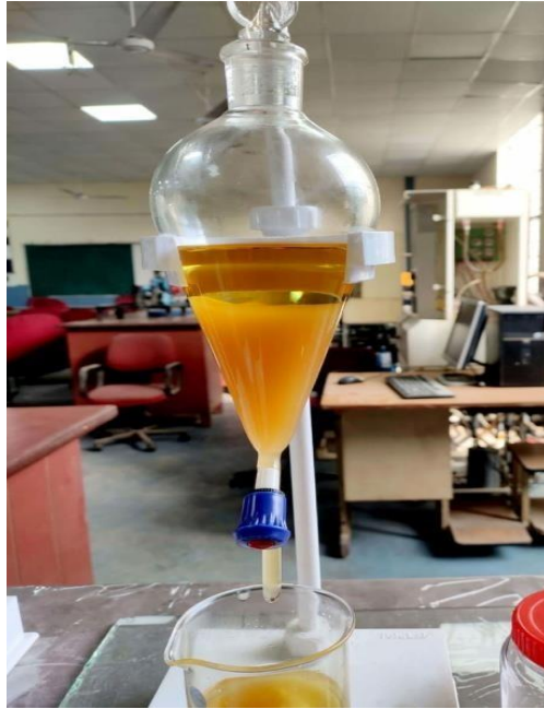
Figure 3.2: Separation of biodiesel from glycerol
