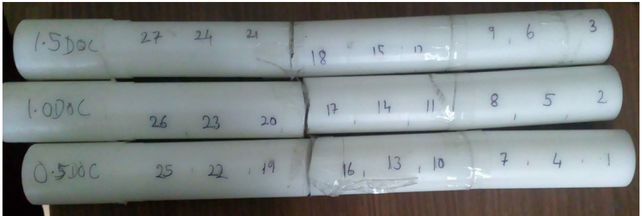
Figure 3.6 Turning operation performed on Delrin rod with different input values
