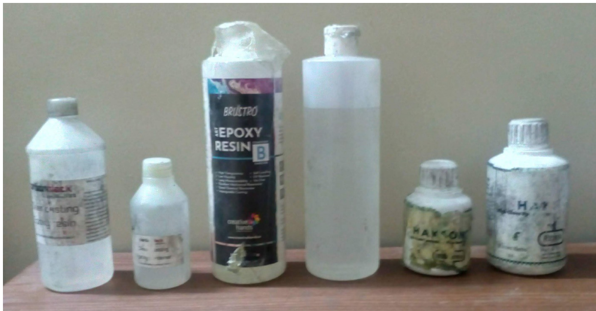
Figure 3.7 (From Left to Right) Resins and Hardeners of ratios 2:1, 5:3, and 3:1.
