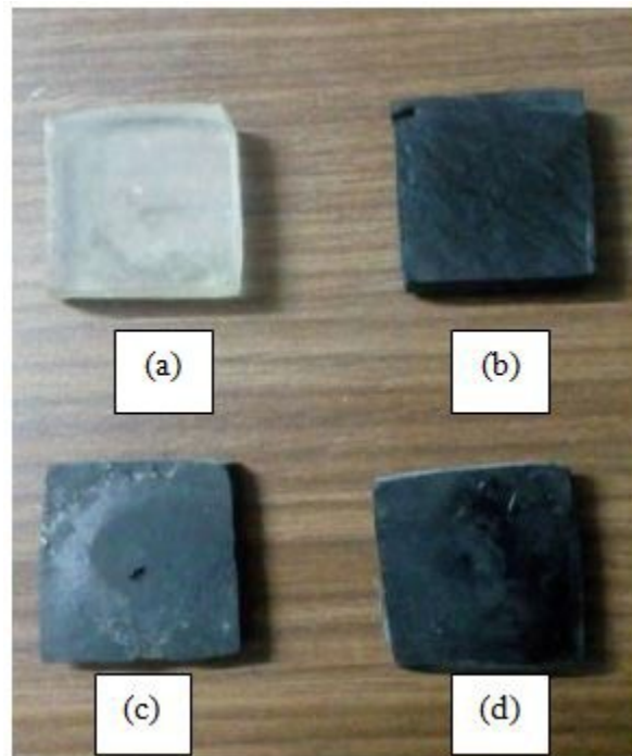
Figure 3.11 (a) Sample L1 without reinforcement, (b) Sample L3 with both RHA and GSA as reinforcements, (c) Sample L4 with GSA as reinforcement, (d) Sample L6 with RHA as reinforcement
