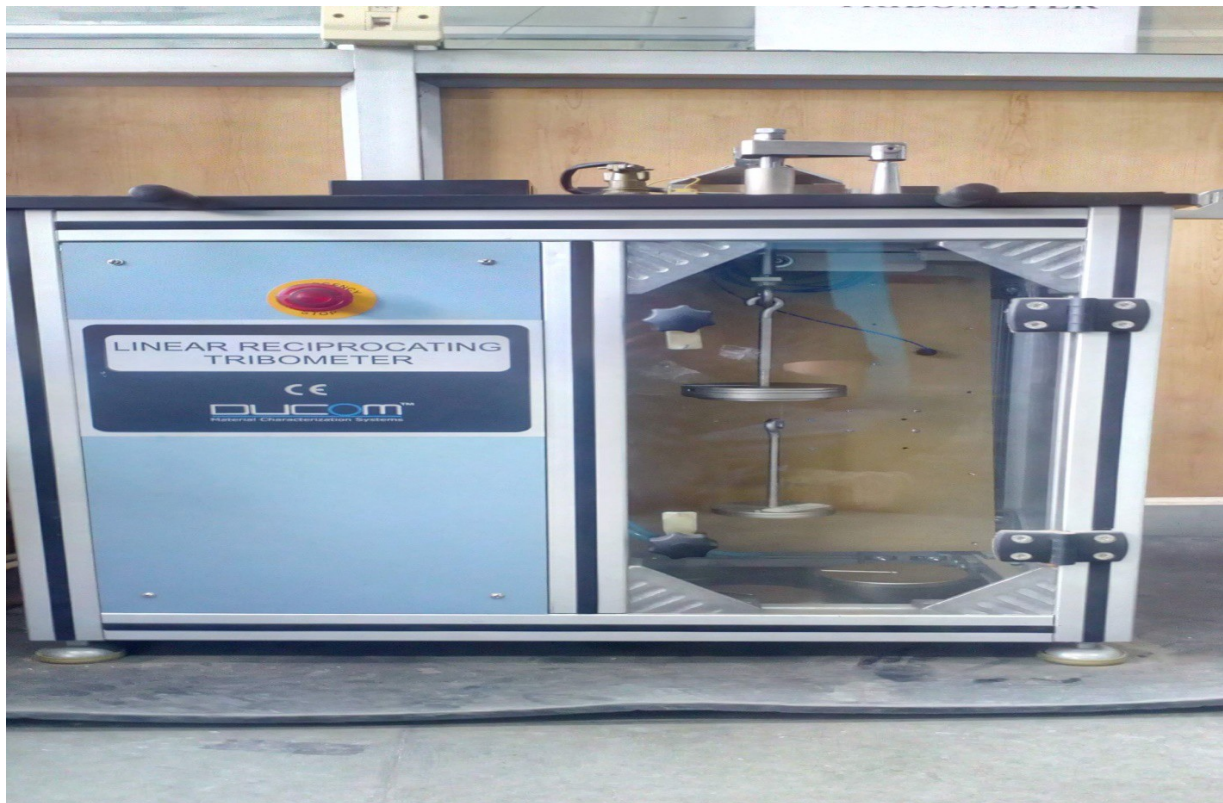
Figure 3.13 Ball on Flat Reciprocating Tribometer (Front View)
