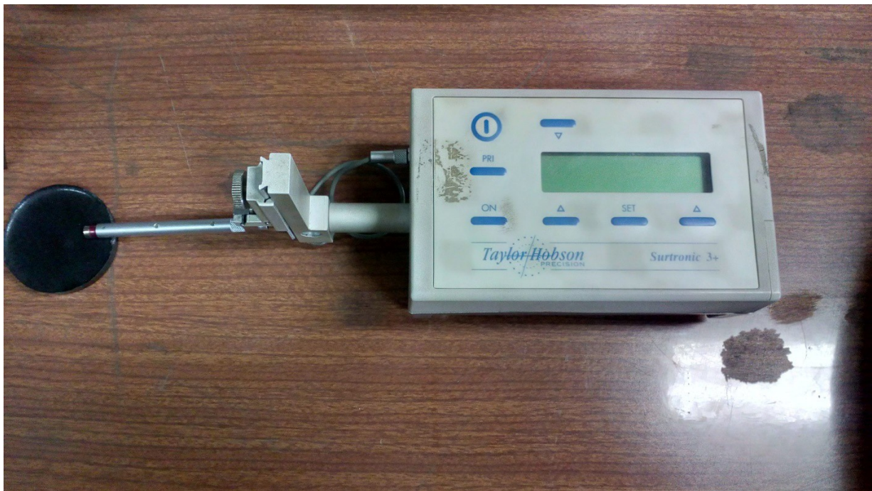
Figure 3.1 Surtronic 3+ surface roughness measuring instrument
