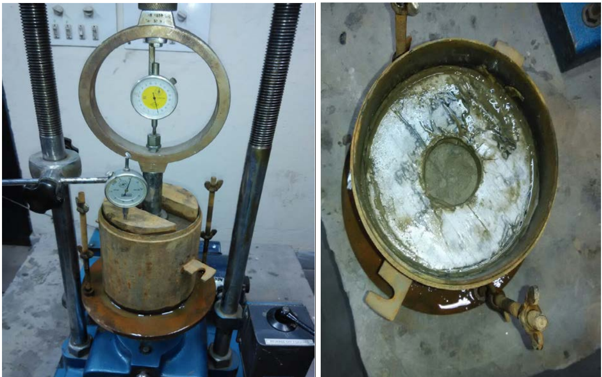
Figure 4.6 CBR test setup and tested sample
