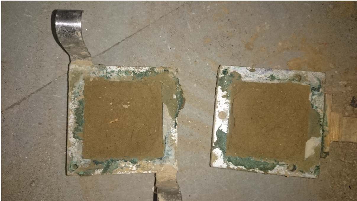
Figure 4.9: Failed sample from direct shear test
