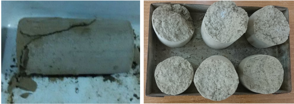
Figure 4.5: Unconfined compression test failed sample
