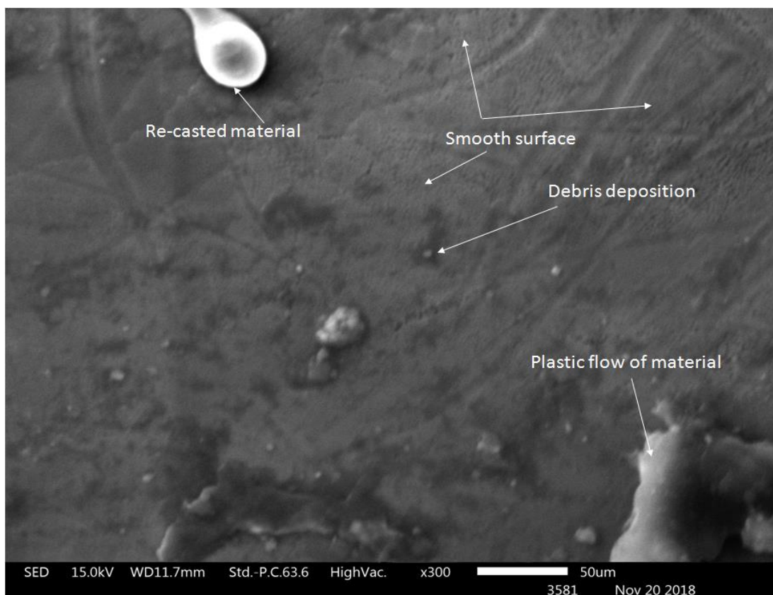
Figure 6.19 (a) SEM Micrograph indicating smooth surface, plastic flow of material
