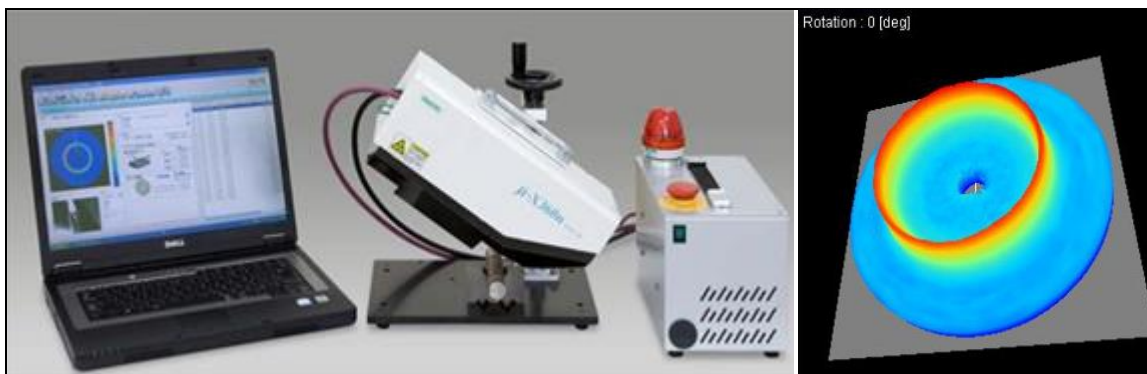
Figure 5.22: Pulsatec \mu - X360 portable stress analyser with Debye-ring
