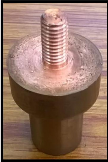
Figure 3.12: Copper tool with threading
