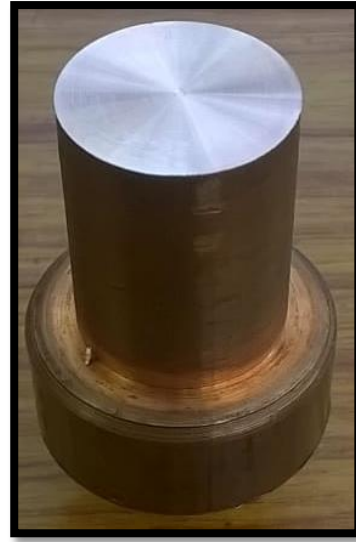
Figure 3.13: Copper tool with facing
