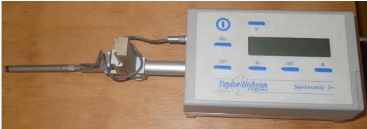
Figure 3.17: Surface Roughness Profilometer Tester
