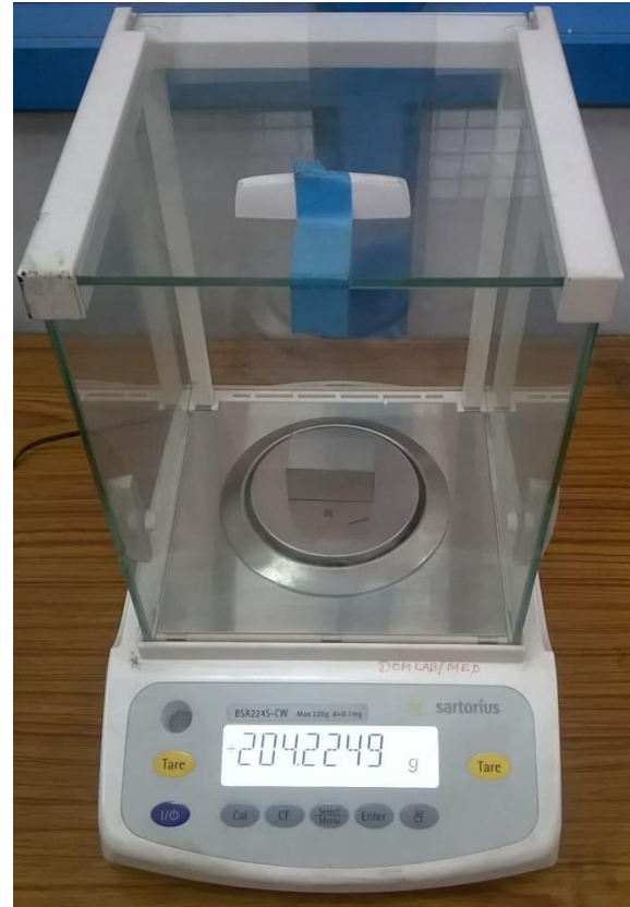
Figure 3.16: Weighing scale for workpiece
