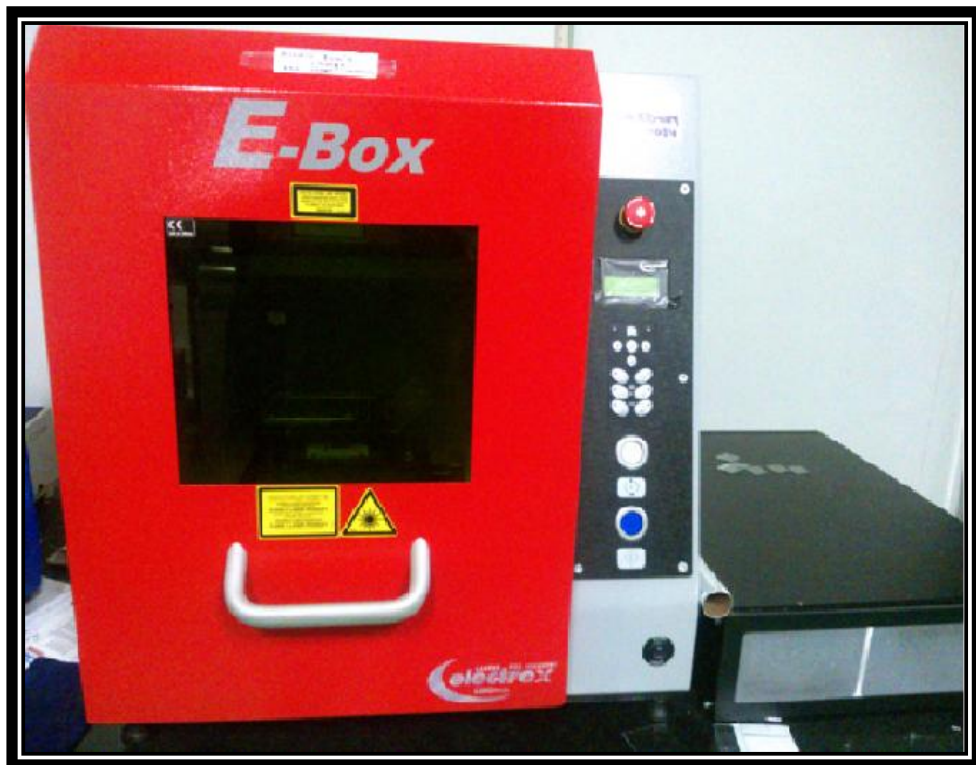
Figure 2.1: Laser scribing machine (Electrox 600 Group, IR L6 1064 nm)
