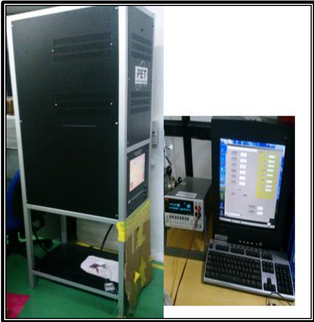
Figure 2.16: A pictorial view of solar simulator (Model SS150AAA) alongwith computer controlled Keithley 2420 source measurement unit
