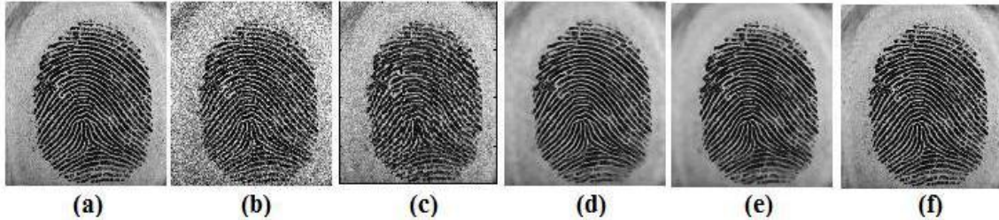
Figure 3.2 Visual performance comparison of different denoising methods (a). Original (b). Noisy (c). K-LLD (d). K-SVD (e). NLM (f). Our Method
