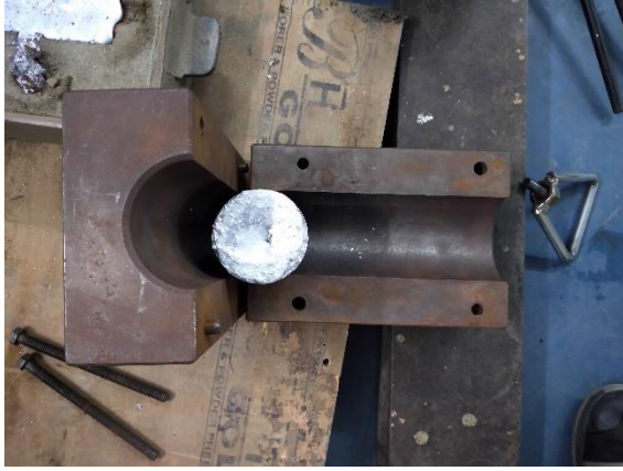
Fig. 4. Sample Preparation using Permanent Die
