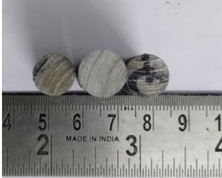
Fig. 6. Microhardness sample cut by Wire EDM
