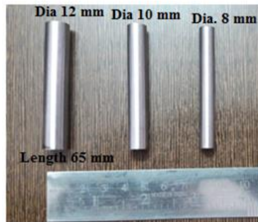
MS PIN USED FOR TESTING
