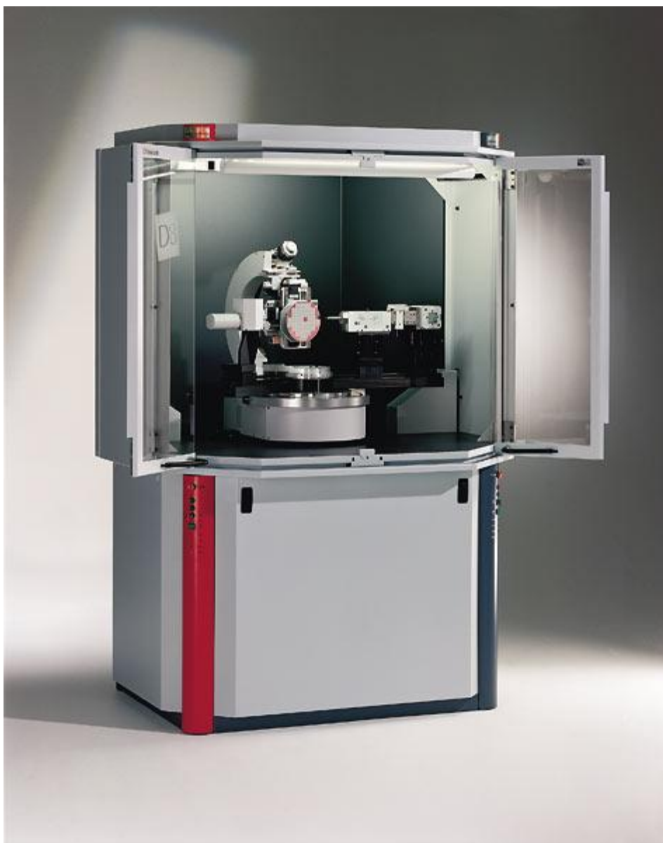
Fig 3.4. Set up used to measure XRD patterns of LTO.
