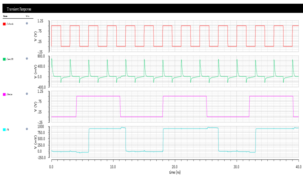
Fig.3.7 Timing waveform of CDFD schematic with 4 TPG
