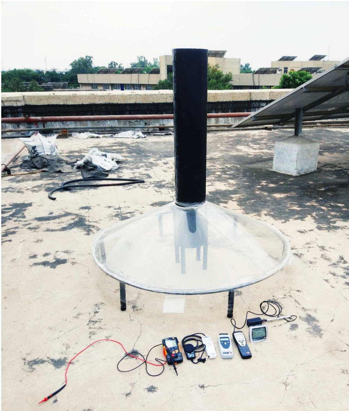
Fig 3.2: Experimental model of SCPP along with the instruments used.
