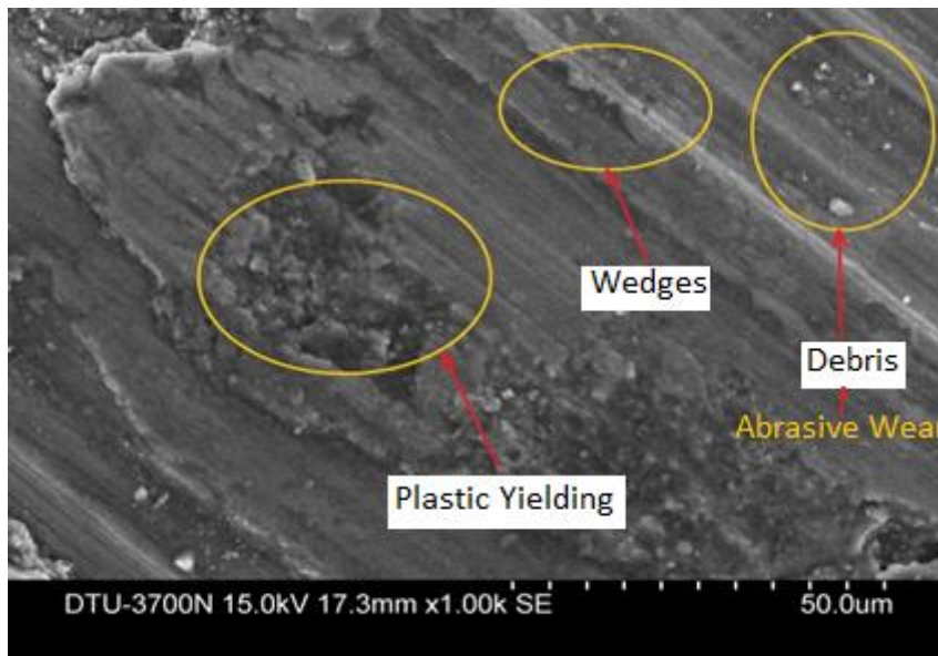
Figure 4.5 (b): SEM images of 4% flyash sample after wear test
