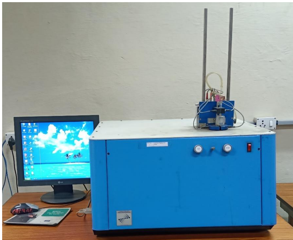
Plate 3.7. The instrument used for measuring CFPP
