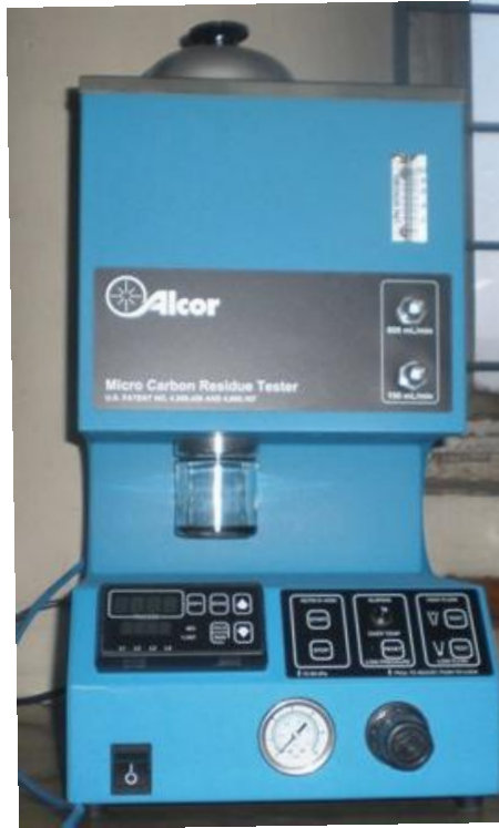
Plate 3.13. Equipment used to determine carbon residue
