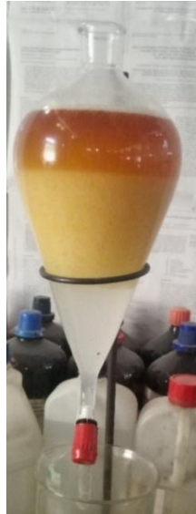
Plate 3.2. Separating funnel showing water washing process
