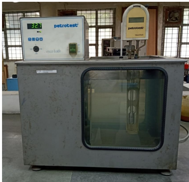
Plate 3.5. The instrument used for measuring Kinematic viscosity
