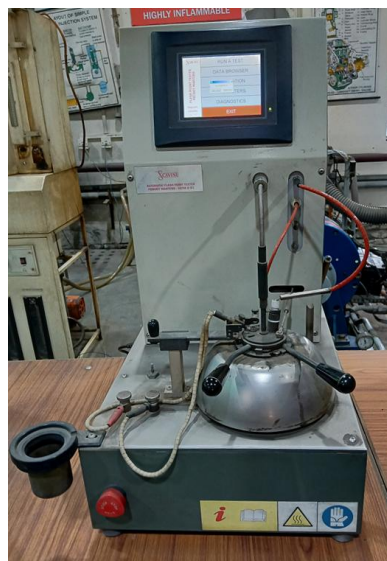
Plate 3.9. Pensky Martens apparatus used for determining flash point
