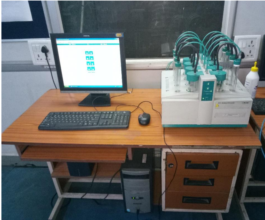
Plate 3.14. The setup used to determine the Oxidation stability
