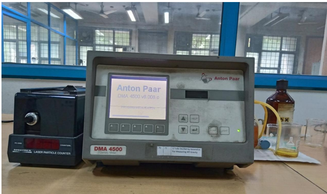
Plate 3.4. The instrument used for measuring density and specific gravity
