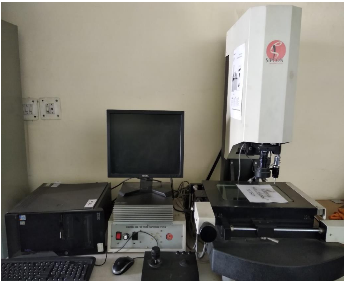
Figure 4.9: Vision Inspection System
