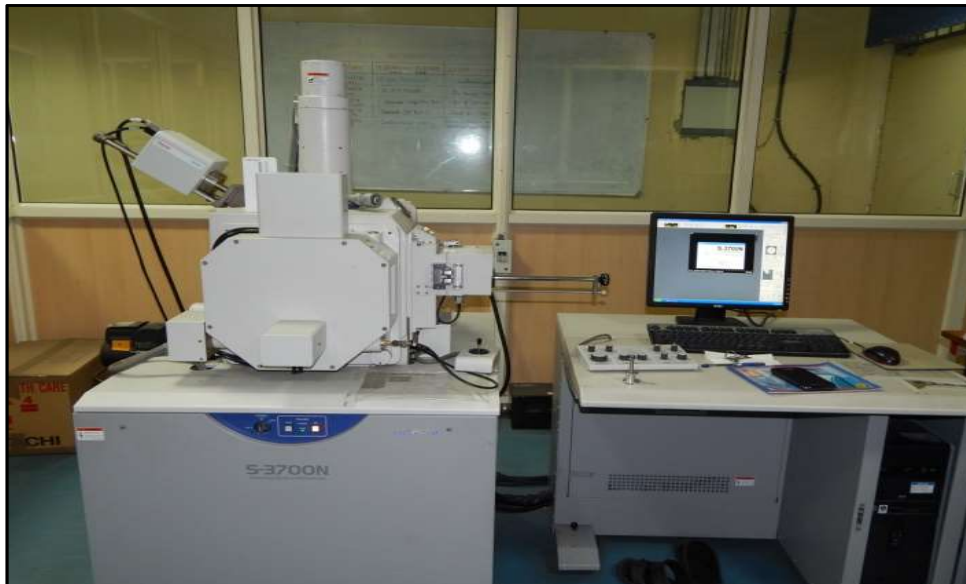
Figure 2.7: Scanning Electron Microscope (Hitachi S-3700N)
