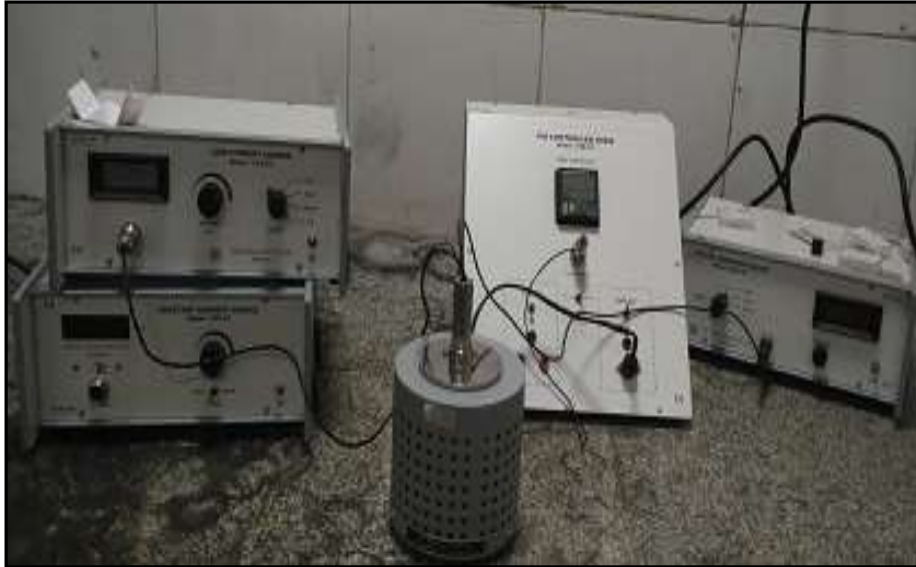
Figure 2.8: Four Probe Digital Conductivity Meter
