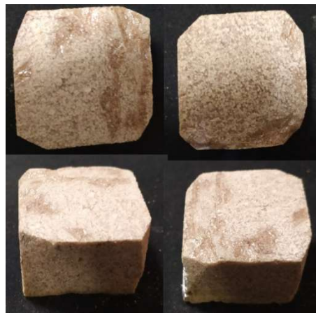
Figure 7.1: Samples Used for Drilling Test
