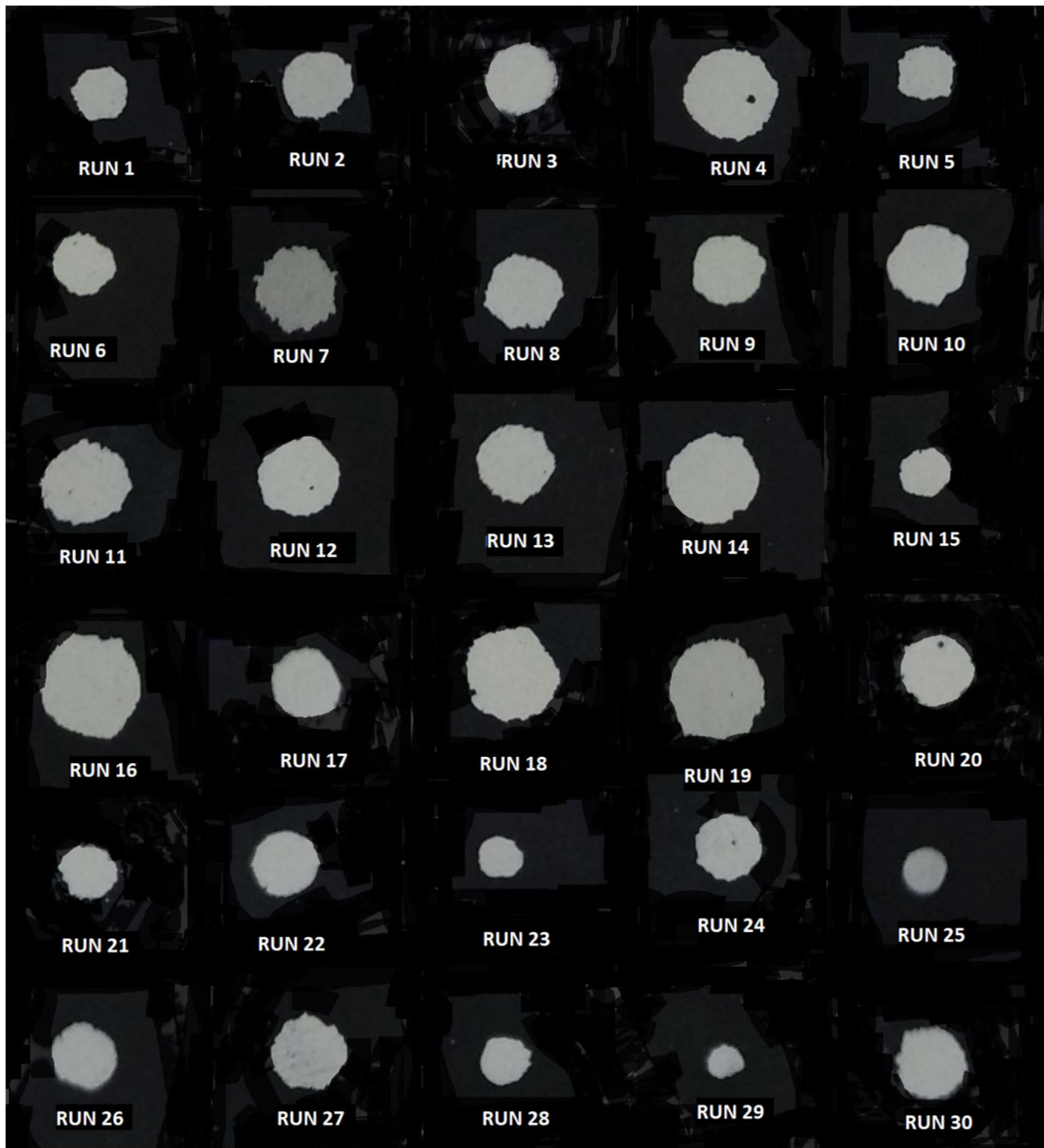
Figure 7.2: Drilled Holes after Performing Drilling Test at Various Factor Levels
