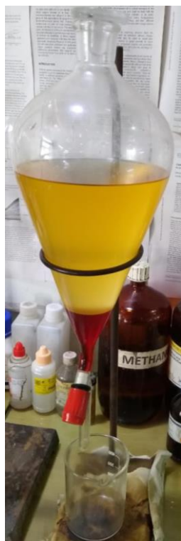
Figure 3.27: Separation of glycerine and biodiesel Figure 3.28: Water washing of biodiesel
