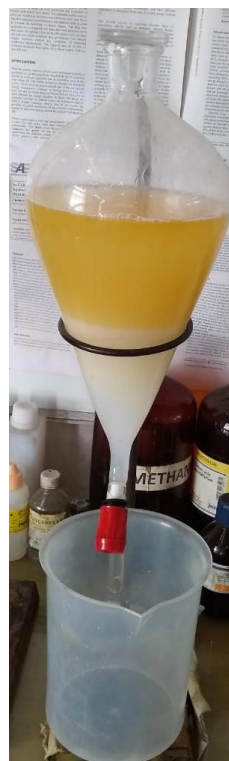
Figure 3.27: Separation of glycerine and biodiesel Figure 3.28: Water washing of biodiesel
