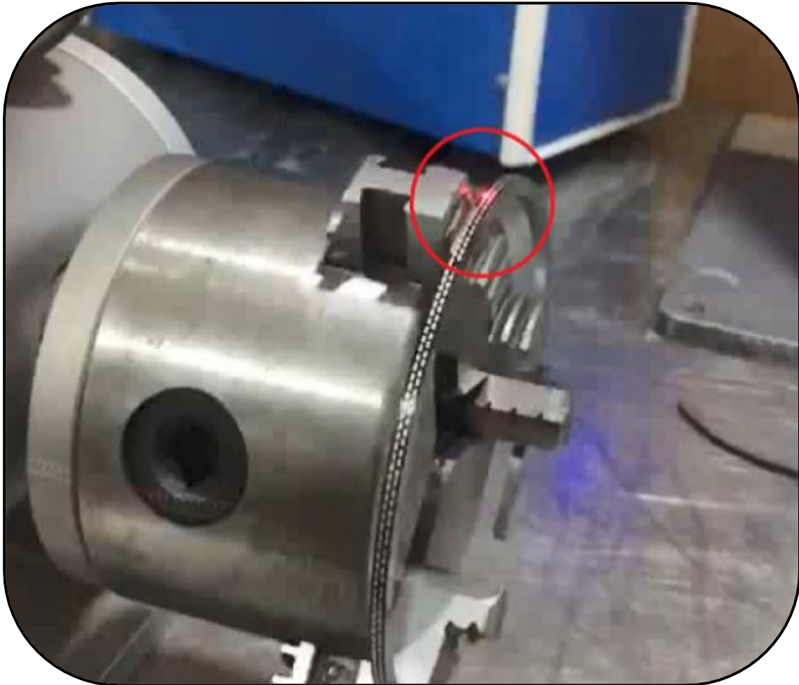
Figure 3.11: Red light being incidental on Piston Ring for laser texturing
