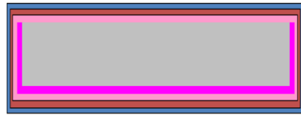
Poly oxidation (0.1 µm)
