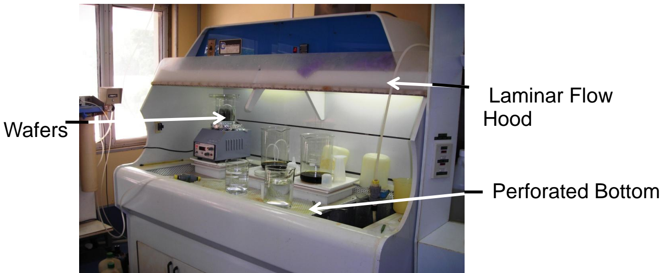
Fig. 6.4 Specialty Chemical Bench for cleaning (RCA cleaning in progress)
