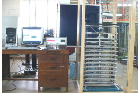
Fig. 2.6 Dead Weight Standard Force Machine (50 N) NPL
