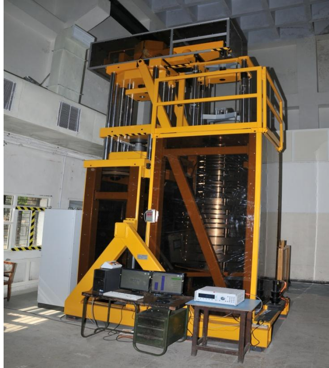
Fig. 2.8 Force Standard Machine (1 MN) at NPL
