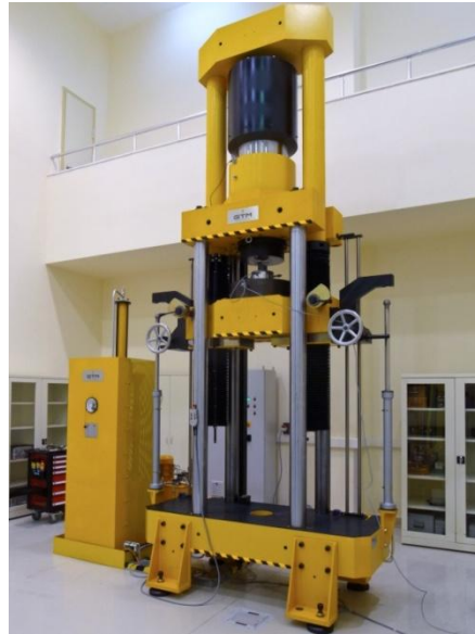
Fig. 2.4 Hydraulic Multiplication Force Machine (3 MN)
