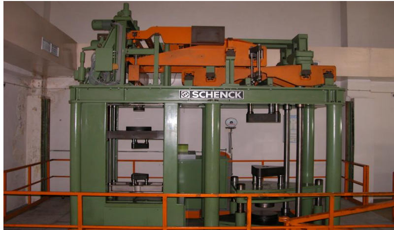
Fig. 2.3 Dead Weight cum Lever Multiplication Force Standard Machine (1 MN) at NPL, India [100]
