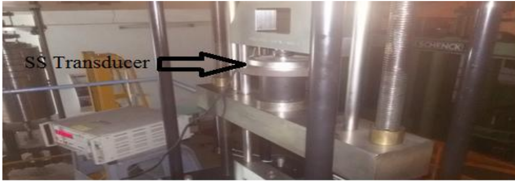
Fig. 5.4 Experimental setup for steel diaphragm force transducer at force machine of 50 kN dead weight at NPL, New Delhi.
