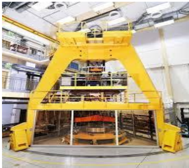
Fig. 2.2 Dead Weight Force Machine (2 MN) at PTB, Germany [95]
