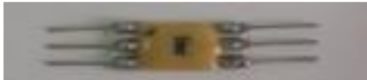
Fig.6.17 Force Sensor packaged on PCB and packed cover with epoxy with open diaphragm
