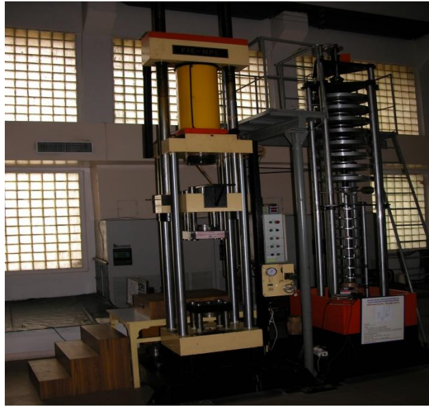
Fig. 2.9 Hydraulic Multiplication Force Machine (1 MN) at NPL
