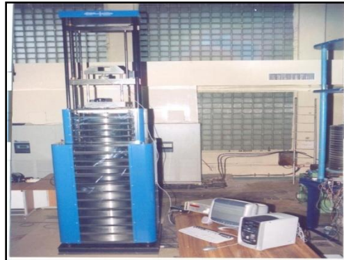
Fig. 2.7 Dead weight Force Machine (50 kN) at NPL [98]
