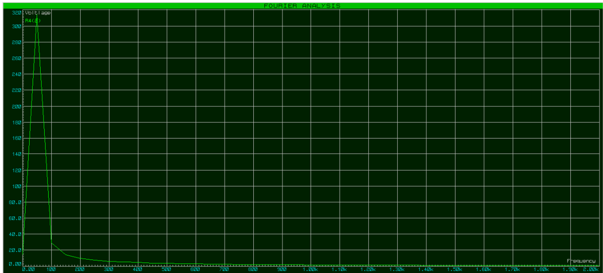
Figure 5.2 Fourier Spectrum of Inverter in 120^\circ conduction mode (with filter)
