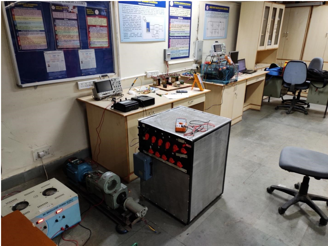
Fig.27. Complete setup for V/f control of induction motor
