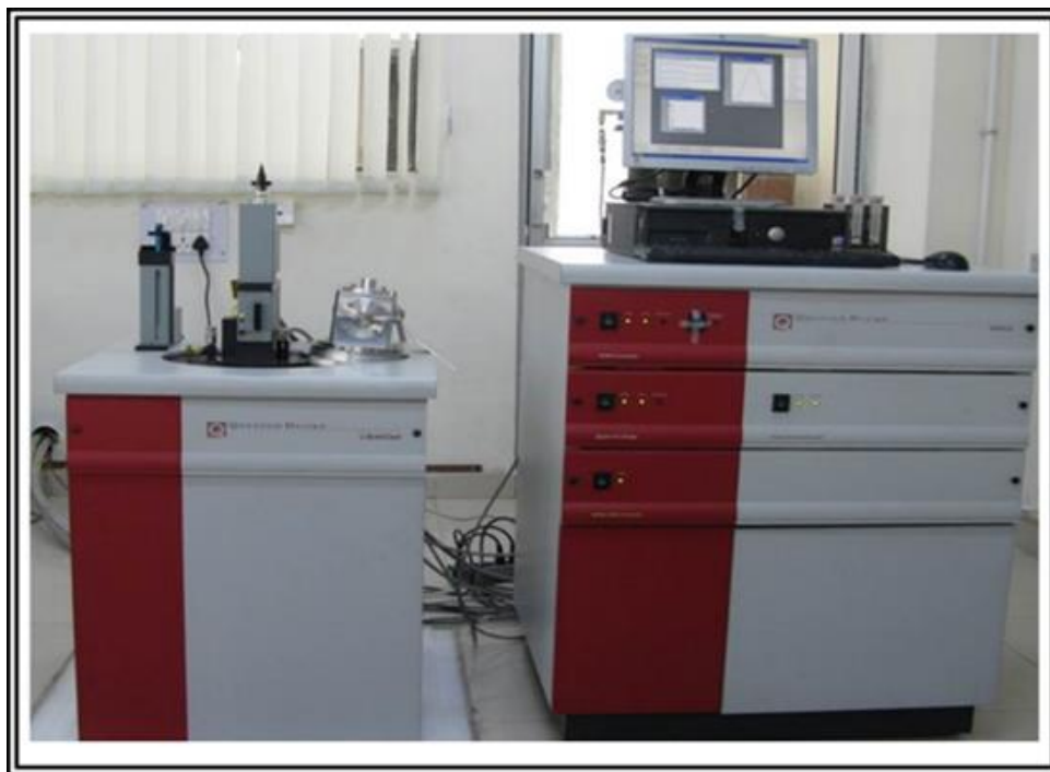
Figure 2.17: The Quantum Design (USA) Magnetic Property Measurement System (MPMS-7T).
