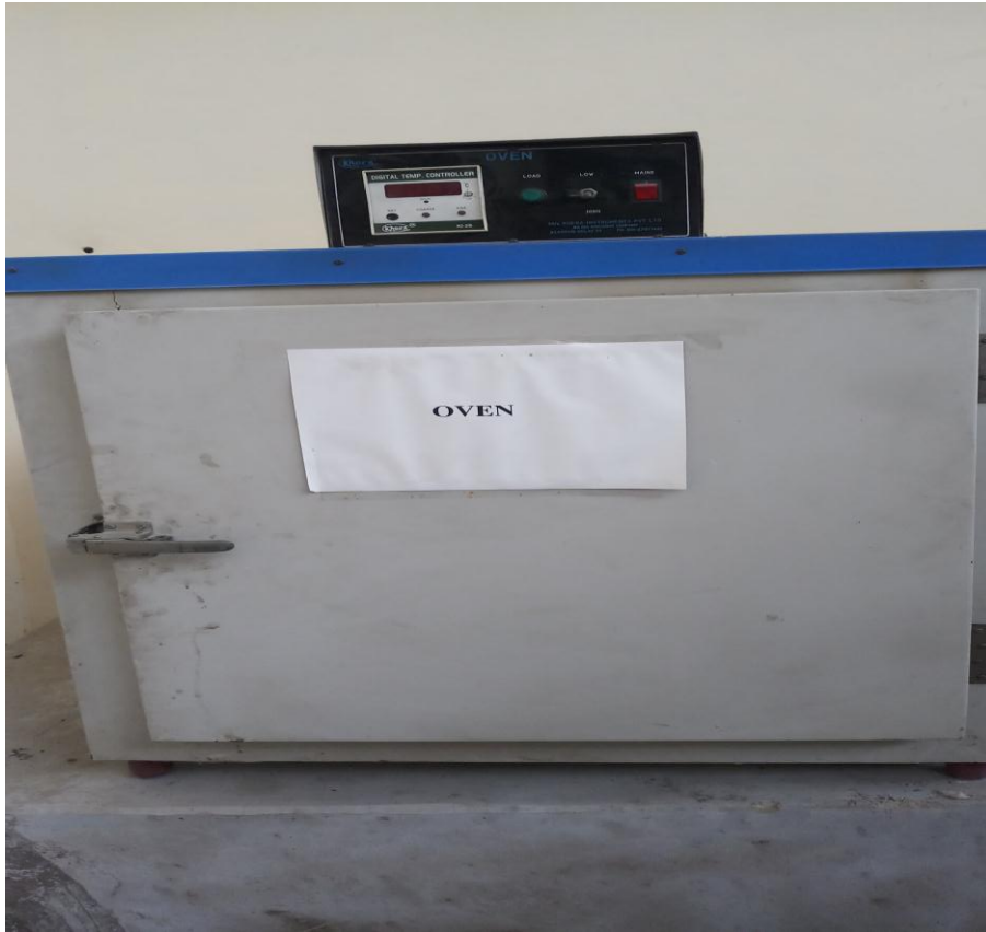
Fig. 3.5 Oven used for curing
