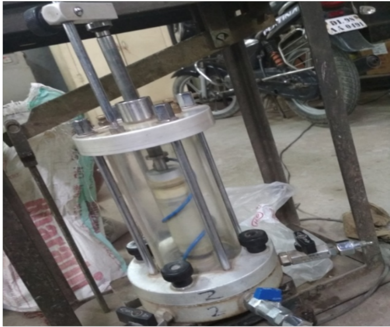
Fig. 4.3 - Triaxial cell with mounted sample
