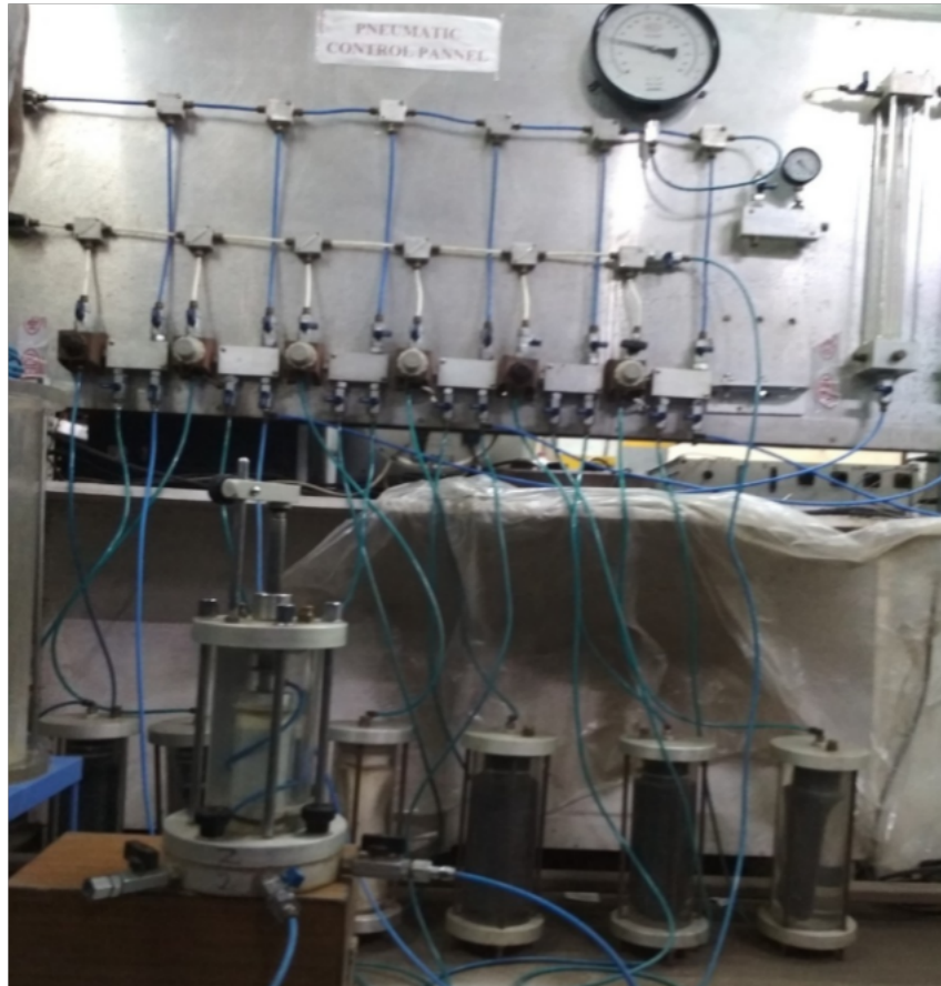
Fig. 4.7 - Triaxial cell connected to pneumatic control panel
