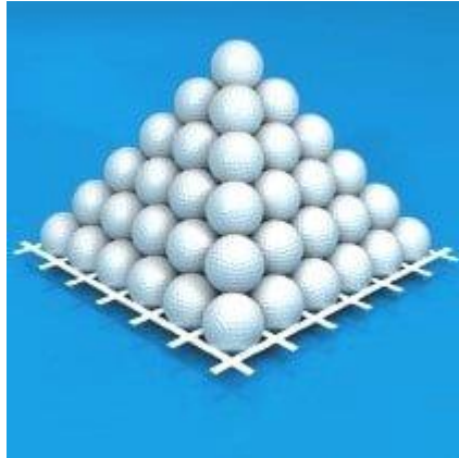
Fig 2.Representation of Geogrid confining the Aggregates (Geotextile Testing and Design Engineer, ASTM STP 952, pp 69116)
