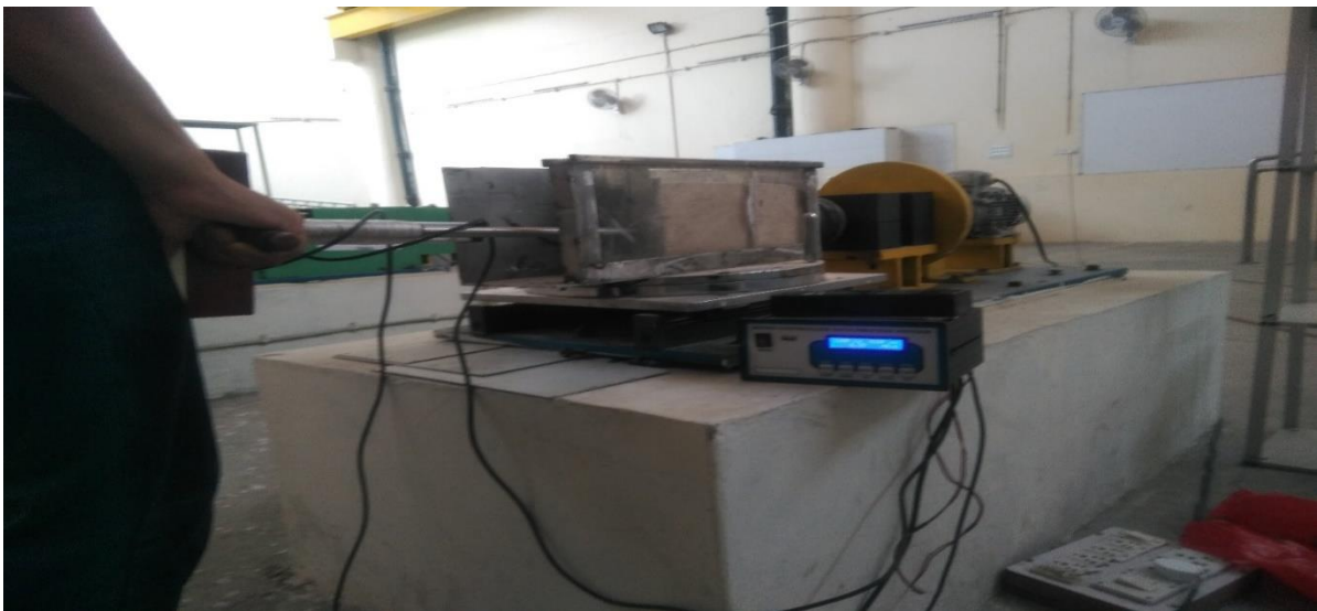
Fig 17: Measurement of Dynamic Displacement of Retaining Wall
