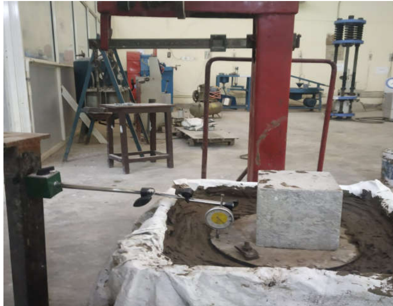
Fig.3.10. Soil after load application
