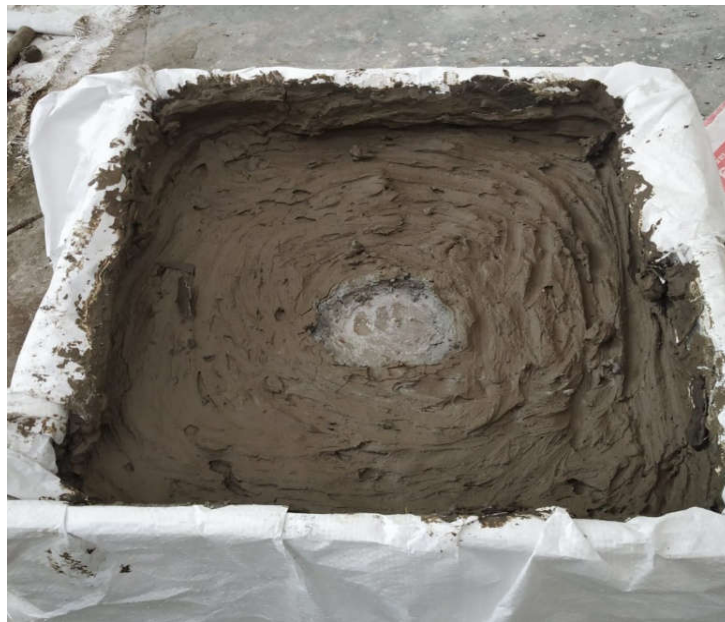
Fig.3.9. Expansive soil with granular column
