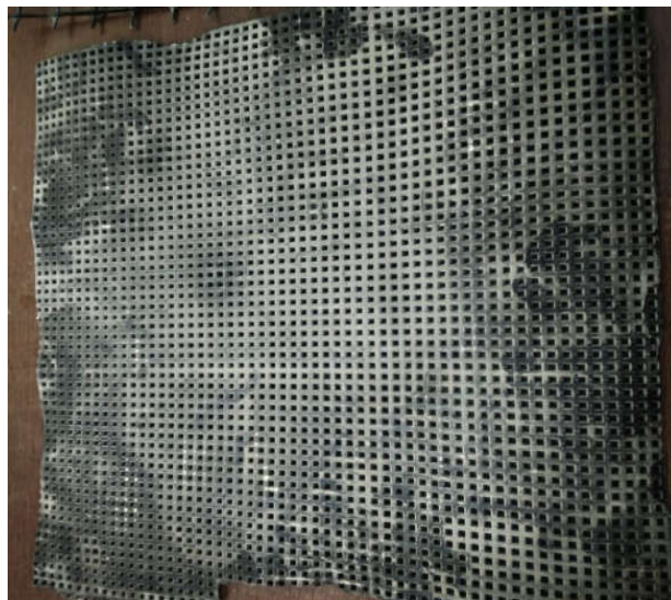
Fig. 3.4 Geotextile used in column
