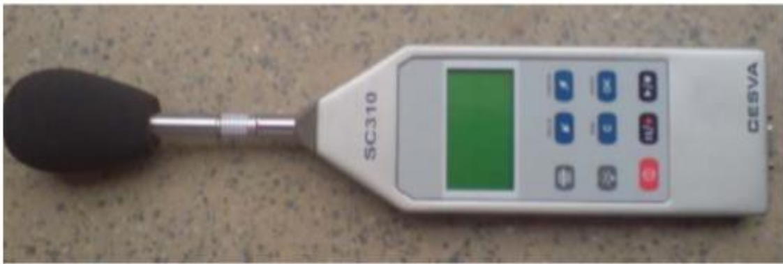
Figure 3.2: Sound Level Meter
