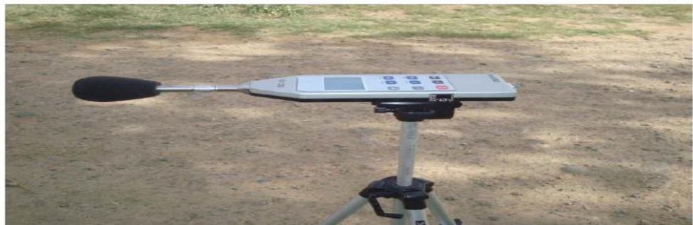
Figure 3.15: Sound Level Meter attached on tripod
