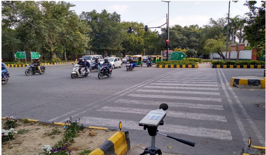
Figure 3.7: Noise monitoring at K.G & Tolstoy Marg
