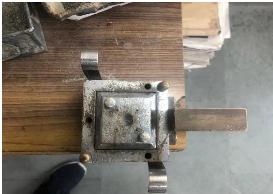
Fig. 3.19 Shear Box Filled with Sand
