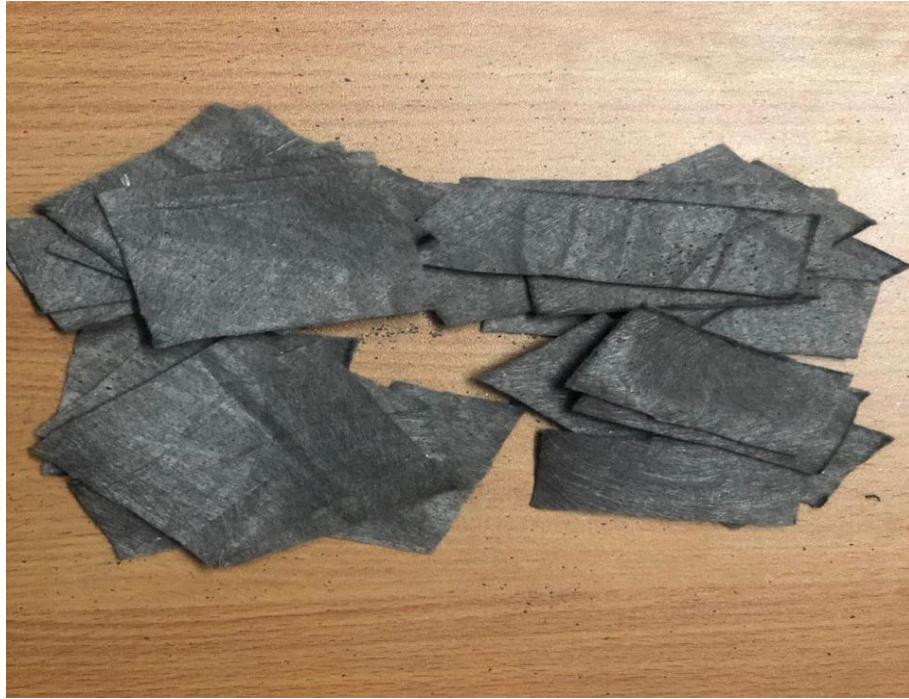
Fig.3.21 Failed Geo-textile Pieces
