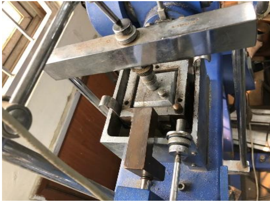
Fig.3.20 Shear Box Placed Inside DSA
