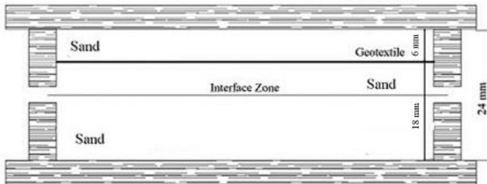
Fig. 3.12 Geo-textile placed at centre of upper part
