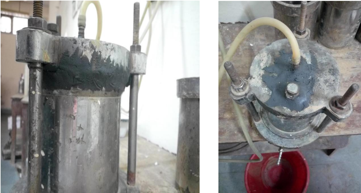
Figure 3.2 Falling Head Hydraulic Conductivity Mould
