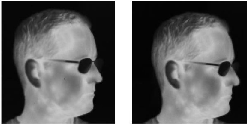
Figure 1.2 Thermal pictures obtained under absolute Dark environment (Left-side) and room brightness (Right-side)
