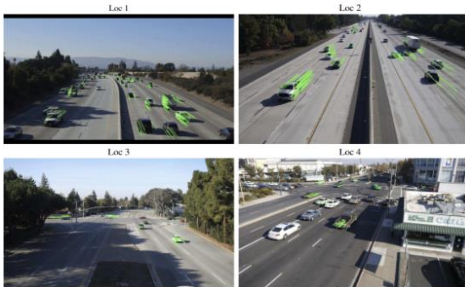
Figure 2.8 : Real-time tracking of vehicles with optical flow. [35]
